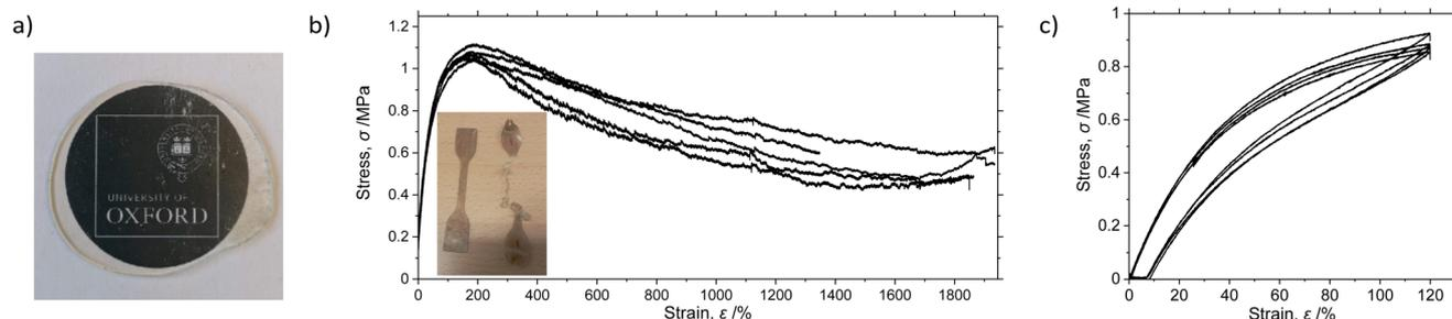
**Fig. 3** (a) Image of pressed transparent disc of UHMWAPP; (b) engineering stress–strain curves (inset: image of dog-bone samples before and after tensile testing), and (c) stress–strain hysteresis curves obtained from UHMWAPP samples.
