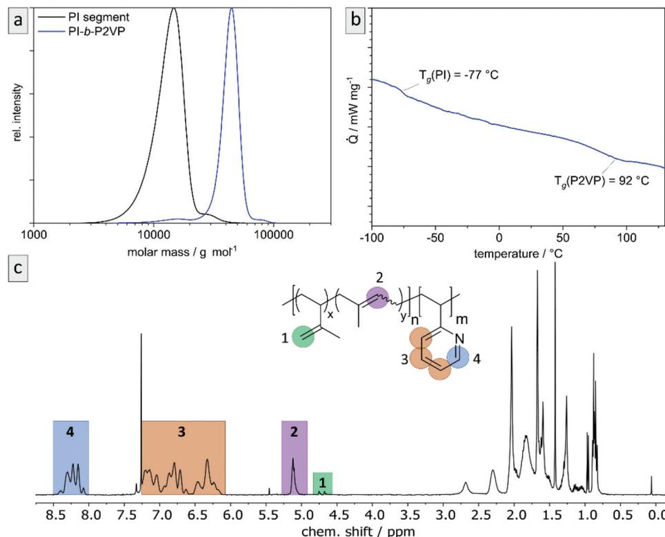
**Fig. 1** Exemplary characterization of  $\text{PI}_{28}\text{-}b\text{-P2VP}_{72}^{63}$  using (a) SEC to determine relative molar masses (vs. PS-standard) and molar mass distributions, (b) thermograms by DSC measurements to determine glass transition temperatures, and (c)  $^1\text{H}$  NMR spectrum in  $\text{CDCl}_3$  to determine chemical composition of BCP and microstructure composition of polyisoprene moieties. For evaluated data see Table 1.
