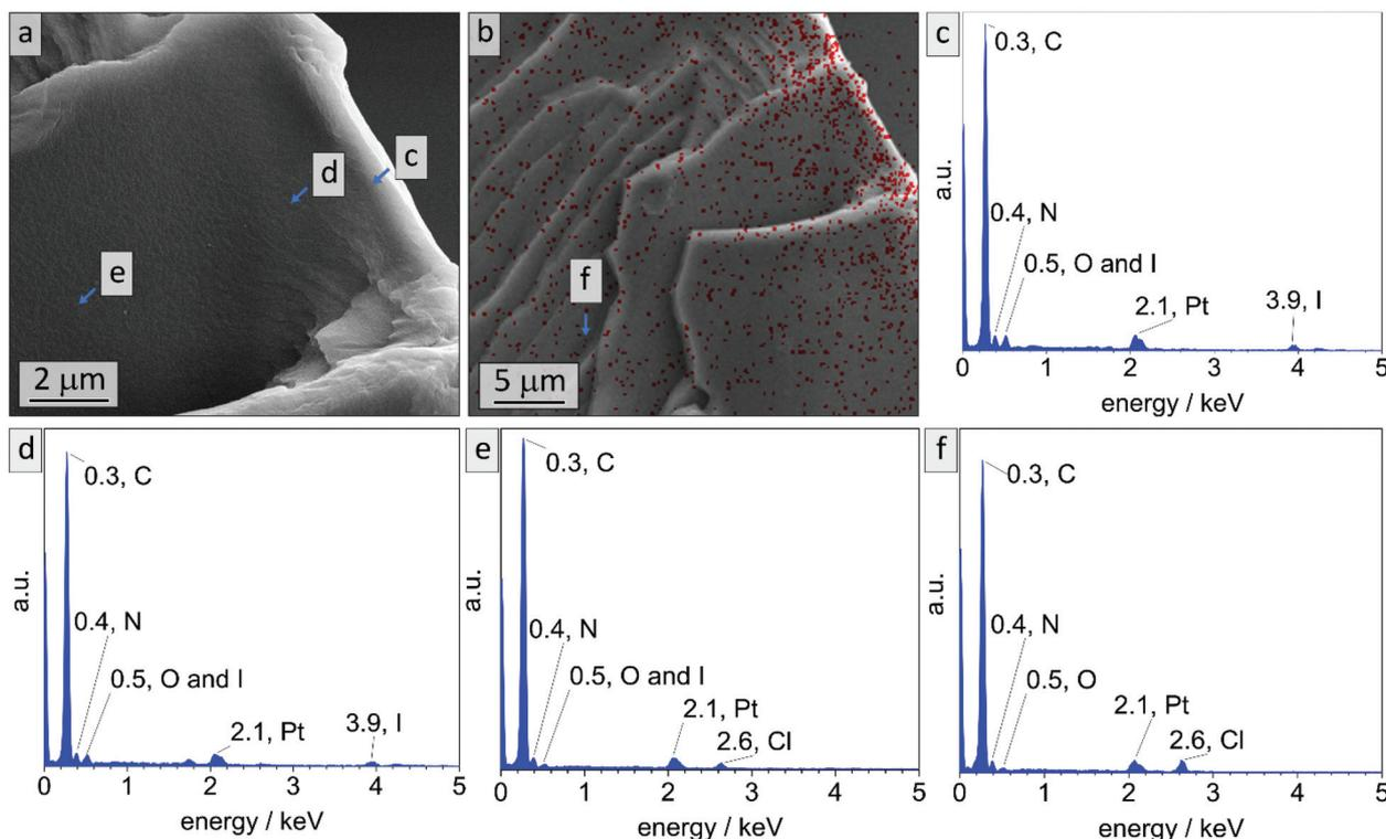
**Fig. 3** EDS data collected on bulk sample  $\text{PI}_{28}\text{-}b\text{-P2VP}_{72}$ <sup>63</sup> after stabilization with DIB. (a) Cross-sectional SEM image, wherein the locations of exemplary EDS point spectra (c–e) are marked. (b) EDS mapping, wherein the location of an exemplary spectrum is shown in (f). The density of red dots refers to relative amount of iodine atoms.
