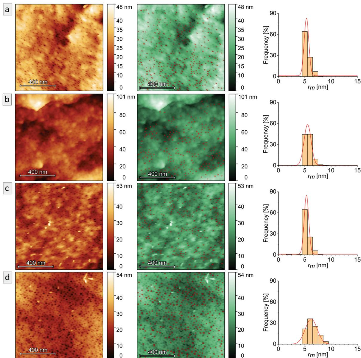
**Fig. 6** AFM images (left, in copper), AFM images masked pores (middle, in green) and the respective histograms (right) of the maximum inscribed radius  $r_m$  with a Gaussian fit (red curve) of each sample: (a) Bs90, (b) B10, (c) Bs10a and (d) Bs10b. All AFM images were obtained in air at 25 °C.
