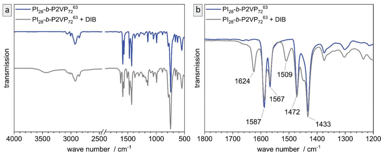
Fig. 4 Analysis of untreated film ( $\text{PI}_{28}\text{-}b\text{-P2VP}_{72}^{63}$ , blue) and DIB-crosslinked film (gray) by ATR-FTIR transmission spectra. (a) overview, whole spectrum, (b) partial spectrum with changes in P2VP signals.
