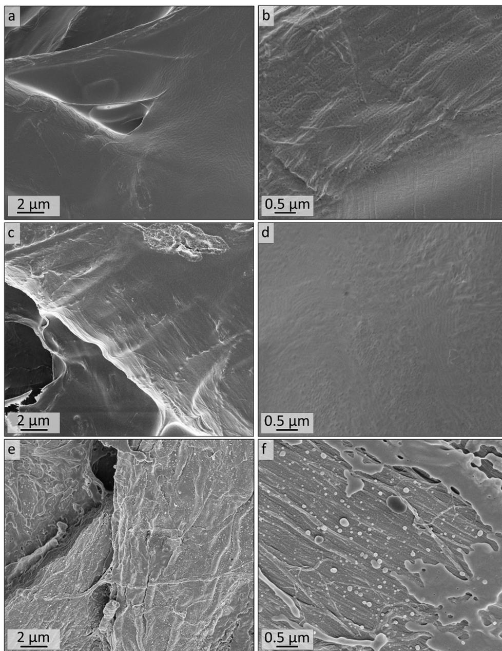
**Fig. 8** SEM analysis of (a and b) the surface of untreated and (c–f) ozone treated composite material using  $PI_{35}$ - $b$ - $P2VP_{65}$ <sup>186</sup> on Munktell cellulose-based filter discs with increasing magnifications. (c) and (d) show the surfaces of the ozone-treated sample Cs10 (DIB-stabilized), (e) and (f) show surfaces of sample C10 (not stabilized).
