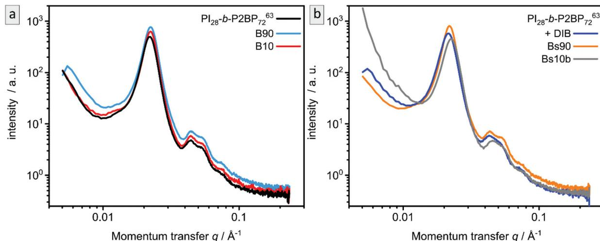
Fig. 7 SAXS of bulk polymer  $PI_{28}\text{-}b\text{-}P2VP_{72}^{63}$  before and after ozone treatment. (a) non-stabilized ( $PI_{28}\text{-}b\text{-}P2VP_{72}^{63}$ ) and ozone treated samples B90 and B10. (b) DIB-stabilized (+DIB) and ozone treated samples Bs90 and Bs10b.
