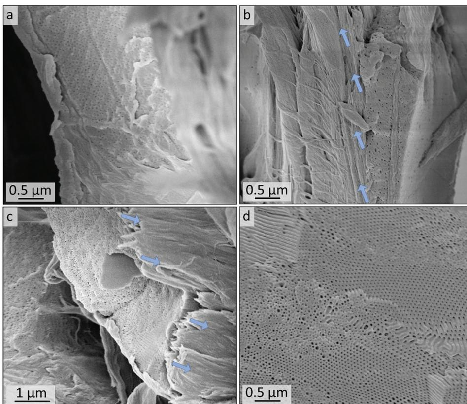
**Fig. 9** SEM analysis of the (a and b) cross-sections of untreated and (c and d) ozone treated composite material (sample Cs10) using  $\text{PI}_{35}\text{-}b\text{-P2VP}_{65}^{186}$  on Munktell cellulose-based filter discs. Blue arrows indicate cellulose fibers.
