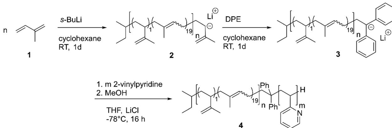
**Scheme 1** Synthetic route leading to polyisoprene-*b*-poly(2-vinylpyridine) (PI-*b*-P2VP) *via* sequential anionic polymerization. Subscripts refer to molar microstructure composition of 1 : 19 for 3,4- and 1,4-linkages, respectively.
