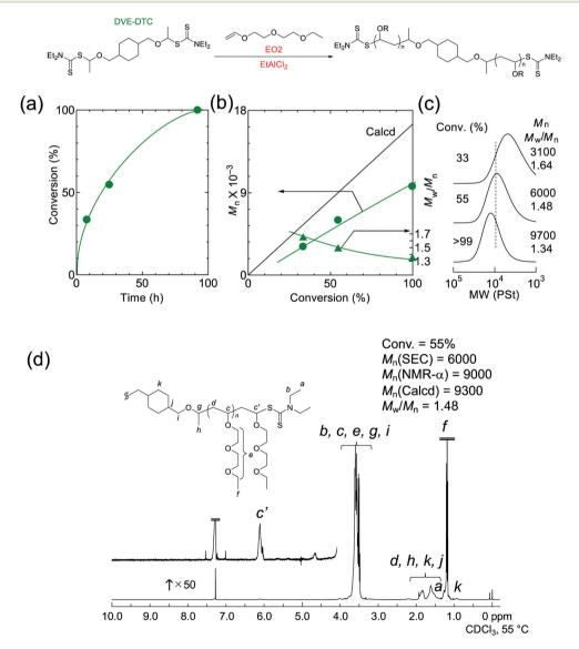
Fig. 3 Living cationic polymerization of EO2 with bifunctional dithiocarbamate (DVE-DTC): [EO2]<sub>0</sub>/[DVE-DTC]<sub>0</sub>/[EtAlCl<sub>2</sub>]<sub>0</sub>/[THF]<sub>0</sub> = 1000/10/15/ 400 mM in toluene at 0 °C. (a) time-conversion, (b)  $M_n$  and  $M_w/M_n$  curves, (c) SEC curves, and (d) <sup>1</sup>H NMR spectrum of the obtained polymer.
