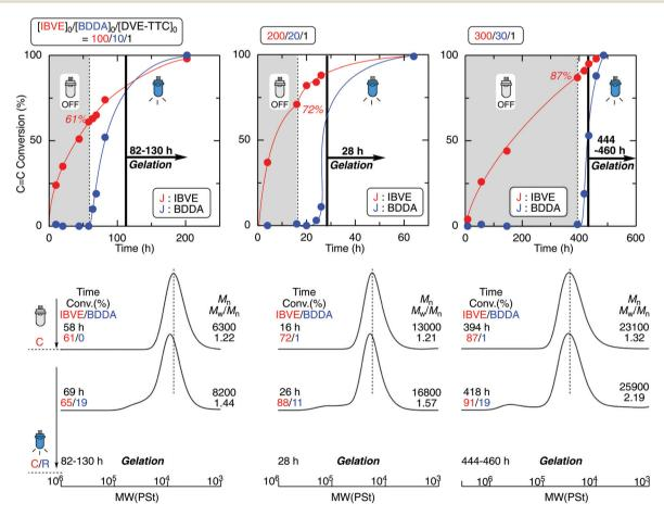
Fig. 1 Mechanistic transformation from cationic polymerization in the dark into cross-linking radical polymerization under photoirradiation: 7.5/2.5/2.5 mM (for 300/30/1) in toluene/Et<sub>2</sub>O (9/1) at 0 °C.
