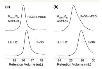
Fig. 6 (a) SEC traces (THF, 35 °C, RI signals, PS standards) of the PRGB precursor and the PRGB-b-PtBGE diblock copolymer (crude products, entry 15 in Table 1). (b) SEC traces (DMF, 50 °C, RI signals, PS standards) of the PRGB precursor and PRGB-b-PEO diblock copolymer (crude products, entry 16 in Table 1).
