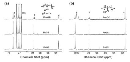
Fig. 3 (a) <sup>13</sup>C NMR spectra (in CDCl<sub>3</sub>) of PRGB, PSGB, and PracGB with a DP of 70 (the isolated products in entries 2, 6, and 10 in Table 1, respectively). (b) <sup>13</sup>C NMR spectra (in DMSO-d<sub>6</sub>) of the corresponding PSGC, PRGC, and PracGC obtained by TBD-catalyzed methanolysis and precipitation
