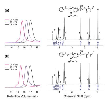
Fig. 1 Left: SEC traces (RI signals, THF, 35 °C) of the crude products of the chemoselective ROP of RGB (a) and SGB (b) with different target DPs (entries 2–7 in Table 1). Right: <sup>1</sup>H NMR spectra (in CDCl<sub>3</sub>) of the isolated PRGB (a) and PSGB (b) with a DP of 30.
