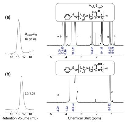
Fig. 4 SEC traces (RI signals, THF, 35 °C, PS standards) and <sup>1</sup>H NMR spectra (in CDCl<sub>3</sub>) of (a) P(PO<sub>50</sub>-co-SGB<sub>50</sub>), corresponding to entry 14 in Table 1, and (b) P(PO<sub>50</sub>-co-RGC<sub>50</sub>) obtained after methanolysis treatment.
