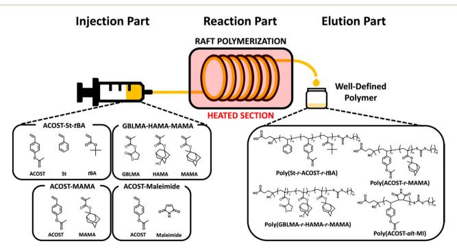
Fig. 1 Schematic of the flow reactor, and structures of copolymers and monomers examined in this study.
