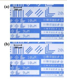
Fig. 9 Optical microscopy images of the photo-patterns fabricated using photoresists consisting of the HNPFBS and poly(HSt-r-MAMA) copolymers synthesized by (a) batch copolymerization and (b) continuous flow copolymerization.
