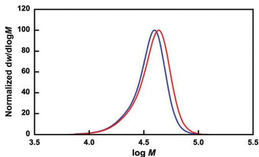
**Fig. 3** Molecular weight distributions (normalized to peak height) of P(OEGMA-co-MEO<sub>2</sub>MA) (blue line) and P(OEGMA-co-MEO<sub>2</sub>MA)-*b*-PMPC (red line).
