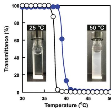
Fig. 7 Changes in transmittance (650 nm) of a PMPC core-shell microgel dispersion in water (●) and an aqueous P(OEGMA-*co*-MEO<sub>2</sub>MA) solution (○) as a function of temperature. (Inserted photos: PMPC core-shell microgel dispersion at 25 °C and 50 °C.)
