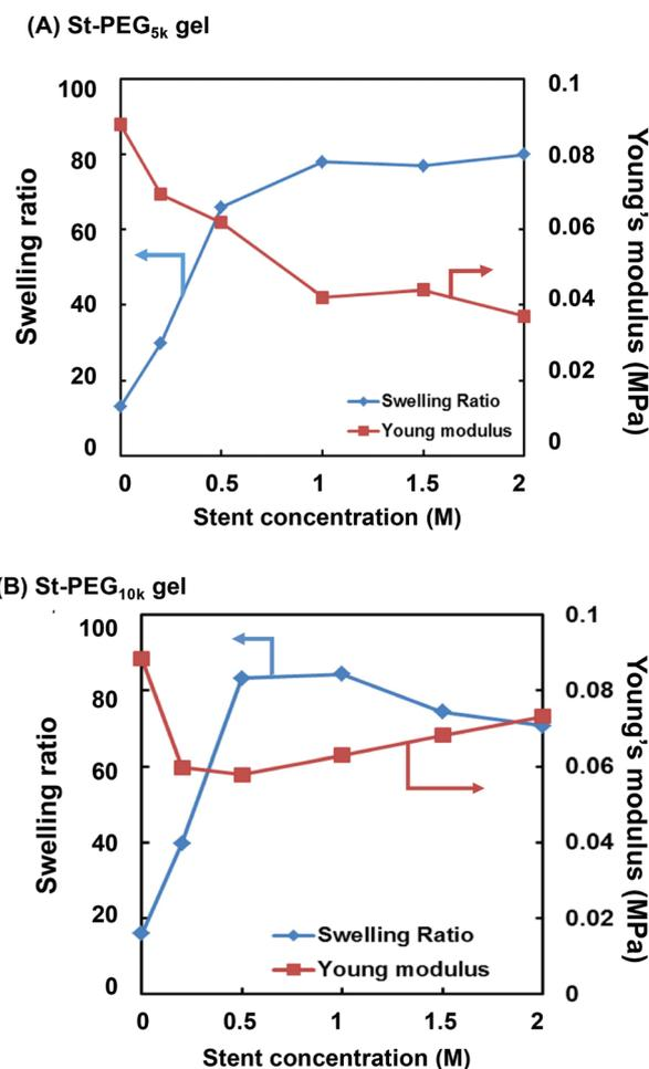
Fig. 4 Effect of stent concentration on the swelling ratios and Young's moduli of the (A) St-PEG<sub>5k</sub> and (B) St-PEG<sub>10k</sub> gels.
