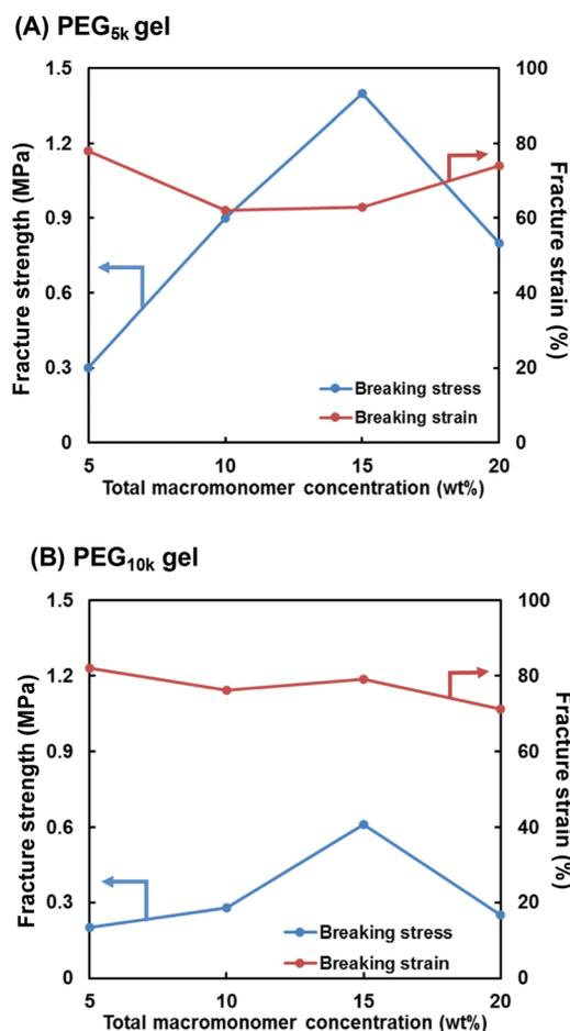
Fig. 3 Effect of total macromonomer concentration (4-arm PEG-SH + PEG-DA) on compressive fracture strength and strain for the (A) PEG<sub>5k</sub> and (B) PEG<sub>10k</sub> gels.
