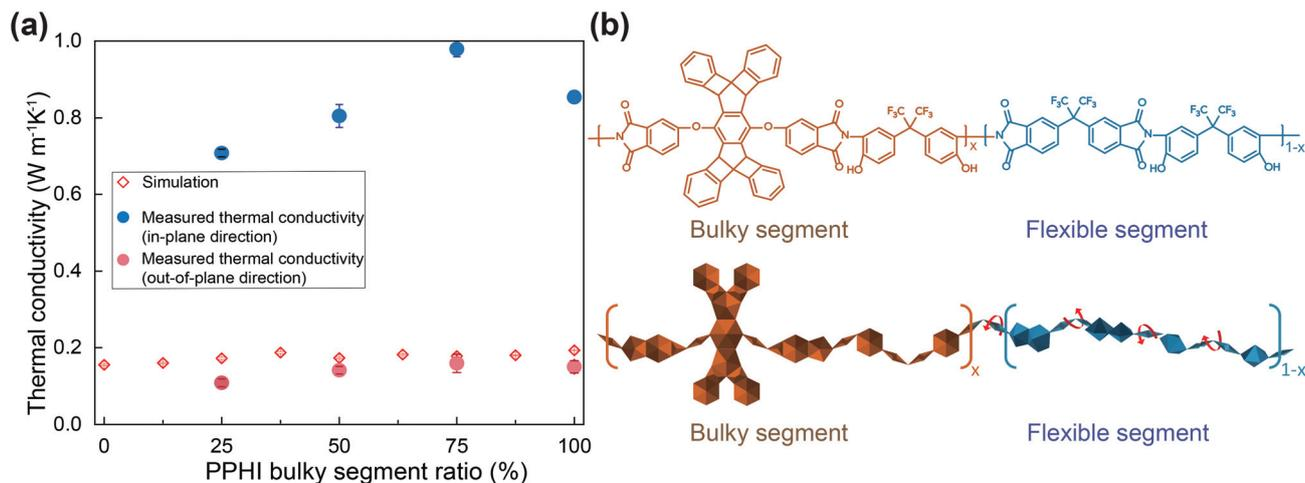
**Fig. 9** (a) Relationships between the bulky segment ratio and thermal conductivity for pentiptycene-based poly(o-hydroxyimide) copolymers. Thermal conductivities are calculated by molecular dynamic simulation (MD simulation)<sup>128</sup> and experimental results for the in-plane direction and out-of-plane direction.<sup>128</sup> (b) Chemical structures of pentiptycene-based poly(o-hydroxyimide) copolymers and schematic of bulky and flexible segments.<sup>128</sup>
