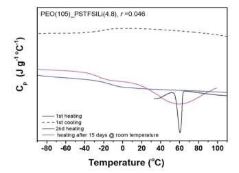
Fig. 7 DSC traces for the PEO(105)\_PSTFSILi(4.8) miktoarm star, with r=0.046. During first heating (black line), during first cooling (black dashed line) and during second heating at 10 °C min<sup>-1</sup> (blue line). The magenta line corresponds to the DSC trace during heating after the sample was left for 15 days at room temperature in an inert environment. The data are shifted vertically for clarity.
