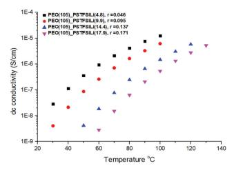
Fig. 9 Ionic conductivity vs. temperature plots, for the synthesized miktoarm star copolymers.
