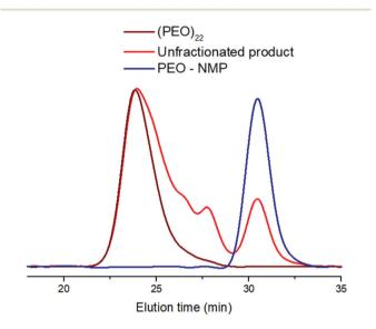
Fig. 2 SEC eluograms, comparing the PEO-NMP, the crude unfractionated product of the cross-linking reaction with DVB and the fractionated star product, (PEO)<sub>22</sub>.
