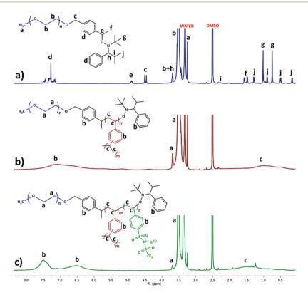
Fig. 1 <sup>1</sup>H NMR in DMSO-d6 spectra of the synthesized PEO macroinitiator (a), PEO star with PDVB core (b), and PEO/PSTFSILi miktoarm star copolymer (c).
