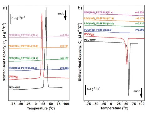
Fig. 6 Cooling (a) and heating (b) DSC thermographs of the linear PEO-NMP (arm precursor, black lines), the  $(PEO)_{22}$  star with PDVB core (red lines) and the PEO/PSTFSILi miktoarm stars with  $r = [Li^+]/[EO] = 0.096$  (blue lines), 0.137 (green lines), 0.171 (orange lines), and 0.204 (magenta lines). The data are shifted vertically for clarity while the black vertical bar indicates a scale of 5 J  $g^{-1}$  C<sup>-1</sup> in heat capacity.
