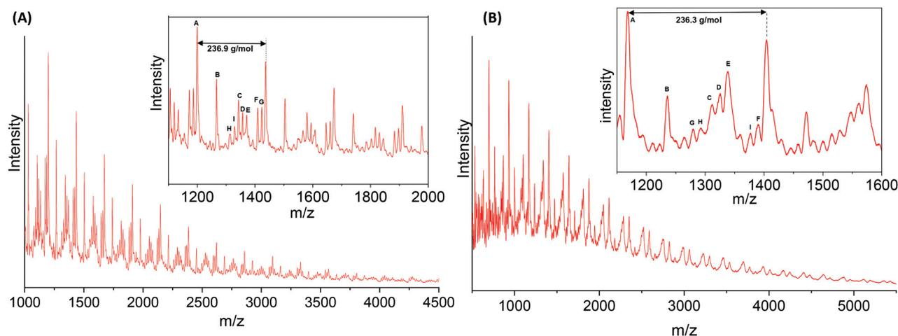
Fig. 7 MALDI-ToF MS spectra for PA6F polyamides synthesised (A) without any catalyst (Table 1, entry 1) and (B) using TIPT 400 ppm catalyst (Table 1, entry 4).
