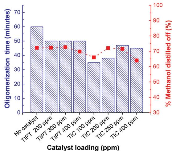
Fig. 3 Oligomerisation step conducted in the presence of both TIPT and TIC at different loadings and uncatalysed reaction. Time needed to reach solid agglomerate formation (blue pattern bars) and amount of methanol distilled off expressed as percentage of theoretical amount to be liberated when reaction goes to completion (red squares).
