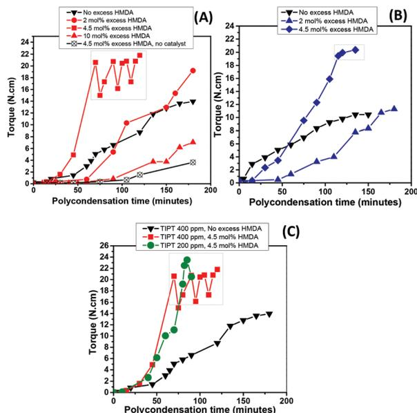
**Fig. 6** Torque versus time plots for the polycondensation step of PA6F synthesised with an excess HMDA using different catalyst loadings (A) TIPT 400 ppm (B) TIC 100 ppm and (C) TIPT 400 ppm and 200 ppm.
