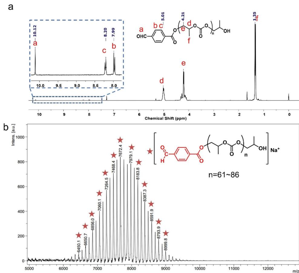
Fig. 3 (a)  $^1\text{H NMR}$  spectrum of aldehyde-end-capped PPC ( $M_n = 10.6 \text{ kg mol}^{-1}$ ) (300 MHz,  $\text{CDCl}_3$ , 25 °C). Inset: Enlarged proton peaks of end groups. (b) MALDI-TOF-MS spectrum of the same sample ( $M_n = 10.6 \text{ kg mol}^{-1}$ ).
