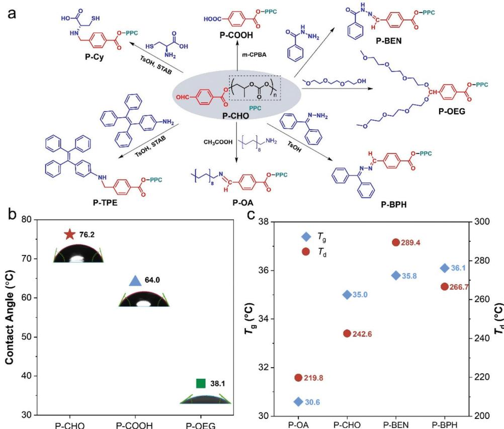
Fig. 4 (a) The synthetic methods of end-functionalized polymers from aldehyde end-capped polycarbonates. (b) The contact angle test of P-CHO, P-COOH and P-OEG. (c) The glass transition temperature ( $T_g$ ) and thermal decomposition temperature ( $T_d$ ) of P-CHO and its post-modified polymers.
