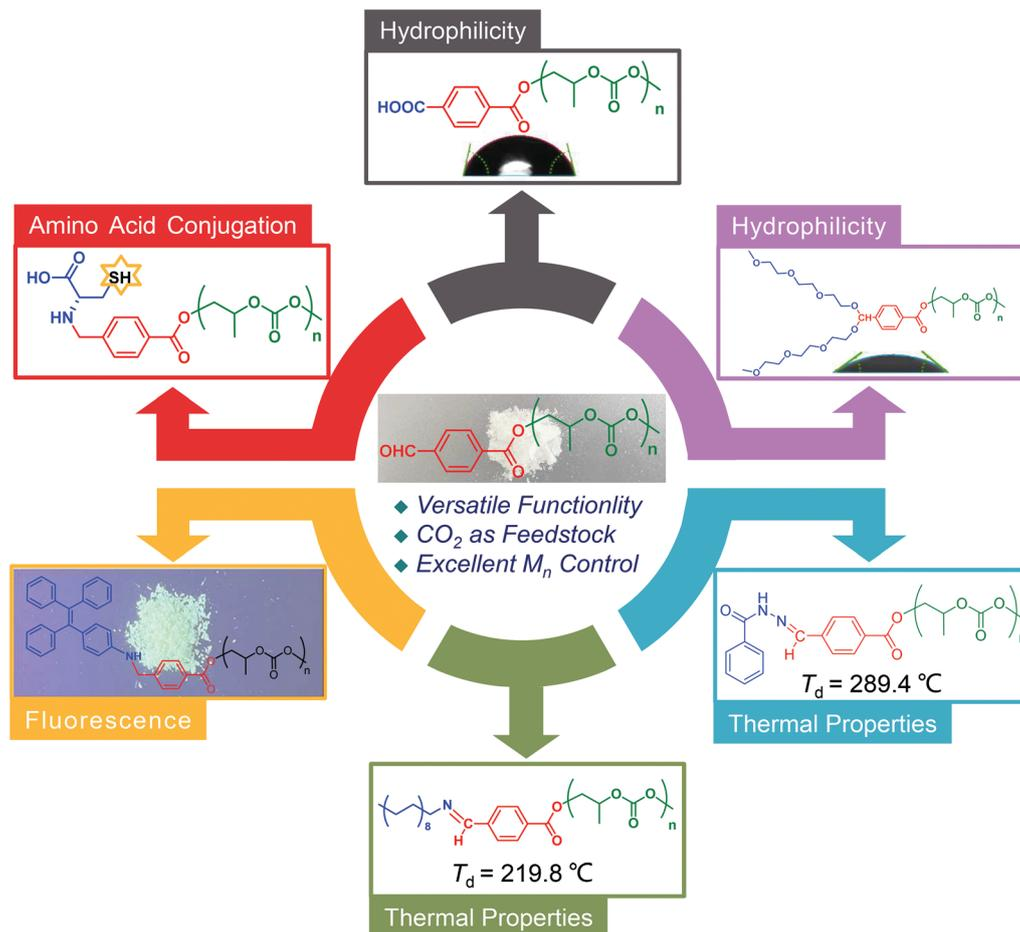
**Scheme 1** Various post-polymerization functionalization routes for aldehyde end-capped CO<sub>2</sub>-based polycarbonates.
