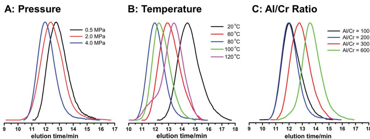
**Fig. 3** GPC curves of polyethylenes prepared from Cr2(THF)/MAO under different (A) pressures (Table 2, runs 1–3); (B) temperatures (Table 2, runs 3–7); (C) Al(MAO)/Cr ratio (Table 2, runs 3 and 8–10).
