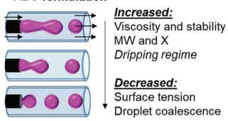
Fig. 2 Through formulation and fluid mechanic optimization, droplet formation shifts from the undesirable jetting regime to the desirable dripping regime.
