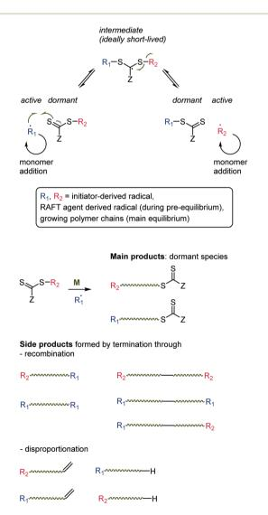
**Scheme 4** Reversible addition–fragmentation chain transfer (RAFT) mechanism (top) and products (bottom).
