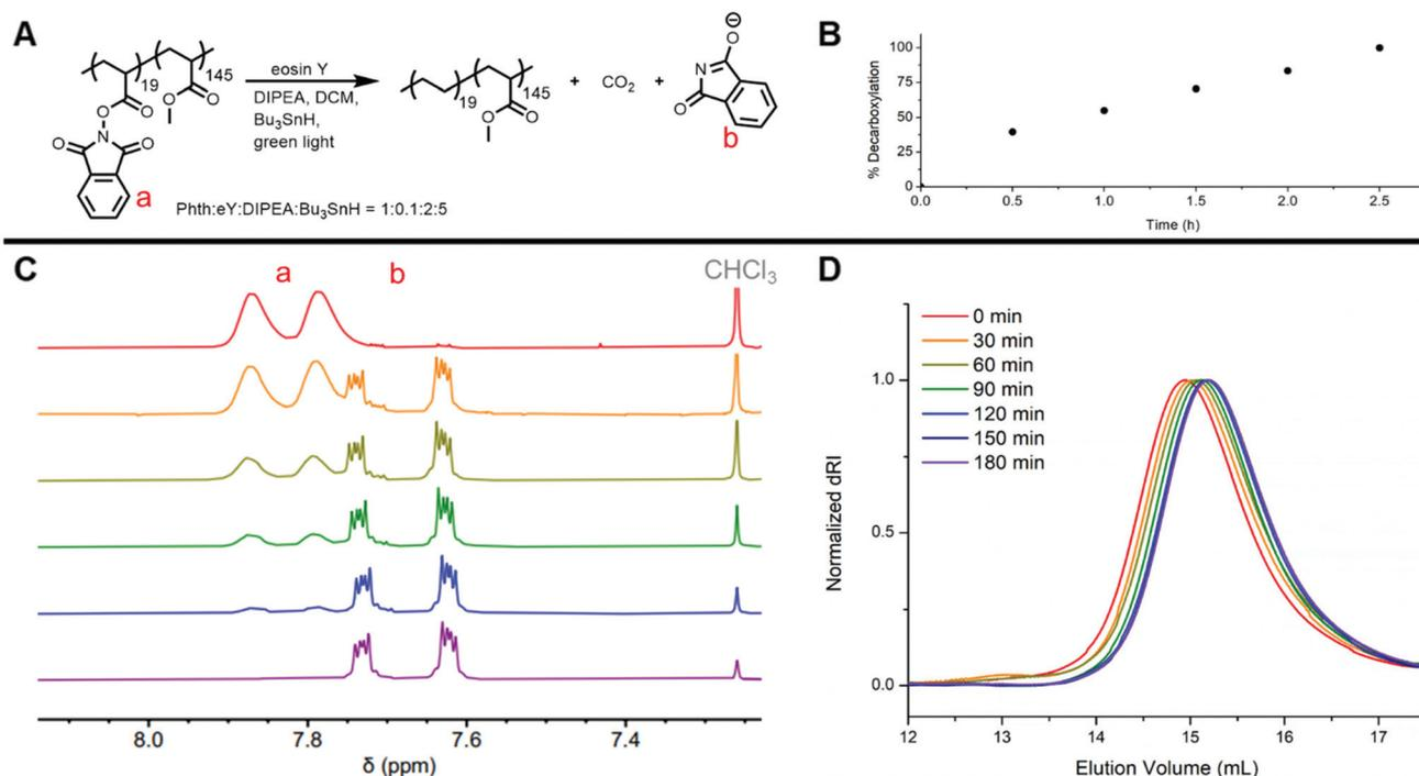
**Fig. 4** (A) Abbreviated scheme for reductive decarboxylation of **RA** (complete proposed reductive decarboxylation scheme in Fig. 2). (B) Decarboxylation percentage vs. time showing quantitative conversion at 2.5 h. (C)  $^1\text{H}$  NMR spectra showing the change in resonance frequency for the phthalimide protons as the reaction proceeded. (D) GPC elugrams showing decrease in polymer molecular weight due to decarboxylation.
