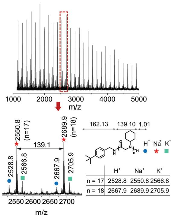
**Fig. 3** MALDI-TOF-MS characterization of polypeptoid prepared from *tert*-butylbenzylamine-initiated polymerization of cyclohexyl-NNCA catalyzed by 5% U-O (molar ratio) in THF at room temperature ( $[M]/[I] = 20$ ,  $[M]_0 = 1$  M). Detailed analysis is shown in Fig. S15.†
