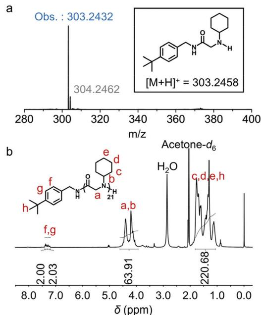
**Fig. 2** (a) HRESI-MS analysis of cyclohexyl-NNCA and *tert*-butylbenzylamine at the molar ratio of 1:1 with 5% U-O (molar ratio) in THF ( $[M]_0 = 0.5$  M). The peak of  $m/z = 304.2462$  belongs to the isotope peak. (b)  $^1\text{H}$  NMR spectrum of polypeptoid synthesized from *tert*-butylbenzylamine-initiated polymerization of cyclohexyl-NNCA catalyzed by 5% U-O in THF at room temperature ( $[M]/[I] = 20$ ,  $[M]_0 = 1$  M).
