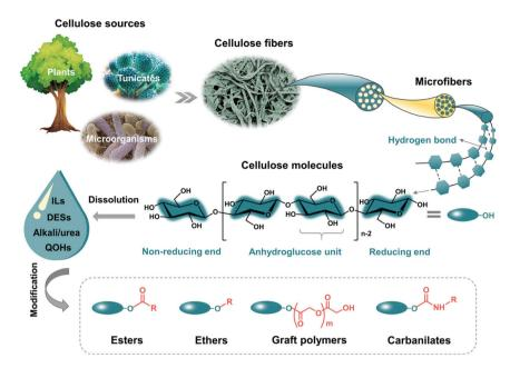
Scheme 1 Structures of cellulose and cellulose derivatives synthesized in green solvents
