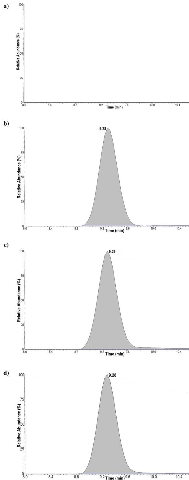
**Fig. 4** Comparative analysis of 4-arylamino-5-hydroxyhexanoic acid **4** and a LGD-4033-positive human urine sample with LC-HRMS in negative ionization mode at the  $m/z$  369: (a) blank, (b) urine-derived sample, (c) synthetic metabolite **4**, (d) co-injection of **4** and urine-derived sample.
