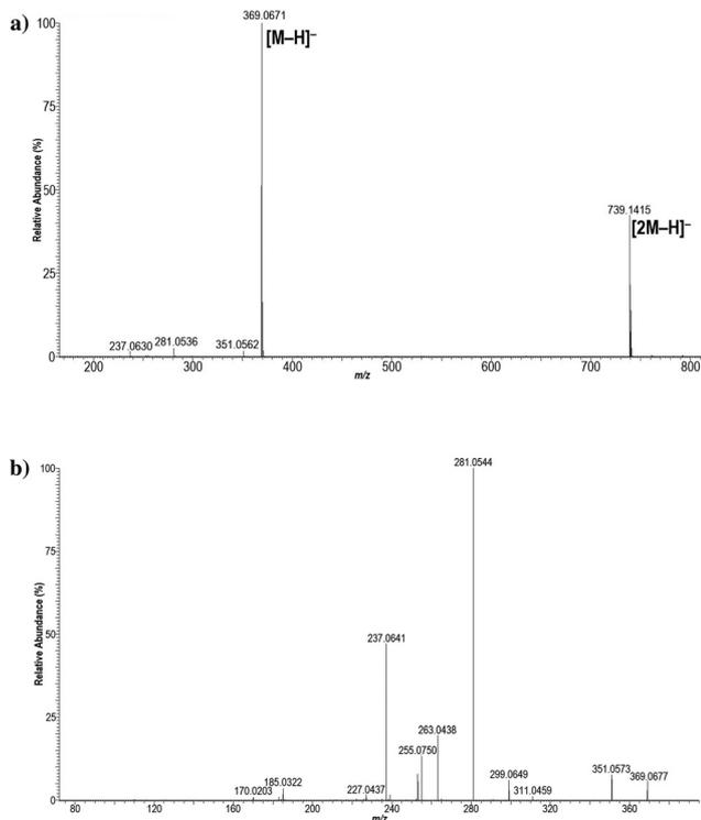
**Fig. 3** Analysis of 4-arylamino-5-hydroxyhexanoic acid **4** with LC-HRMS in negative ionization mode: (a) full scan mass spectrum, (b) product ion mass spectrum of the deprotonated molecular ion  $[M - H]^-$  with  $m/z$  369 at a collision energy of 25 eV.
