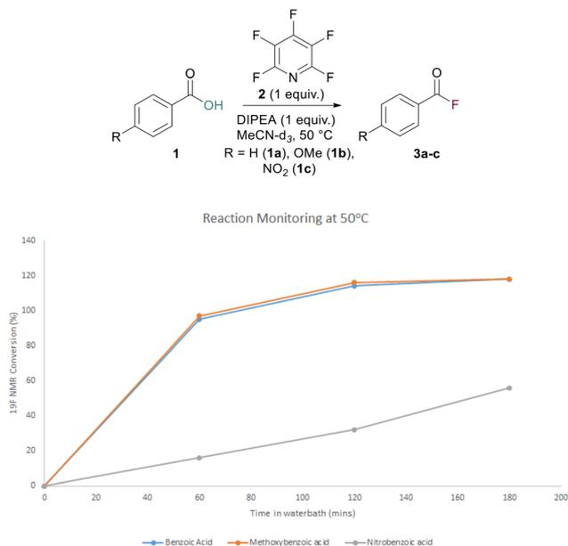
**Fig. 1** Graph of conversion of benzoic acids to acyl fluorides. Reactions were conducted in NMR tubes in a thermostatically controlled water bath.  $^{19}\text{F}$  NMR spectra were recorded at various time points using fluoro-benzene as an internal standard. Integration of the internal standard vs. integration of the acyl fluoride resonance was used to determine conversion.
