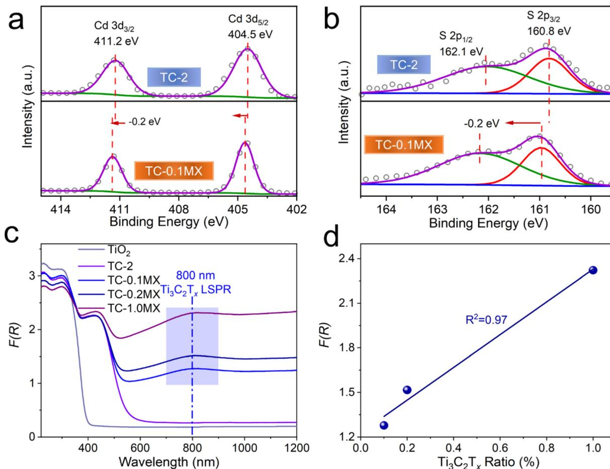
**Fig. 2** XPS spectra of TC-2 (top) and TC-0.1MX (bottom): (a) Cd 3d, (b) S 2p. (c) UV-vis diffuse reflectance spectra (DRS) of the samples and (d) plots of absorption at a wavelength of 800 nm versus the weight ratio of Ti<sub>3</sub>C<sub>2</sub>T<sub>x</sub> in the TC-MX composites.
