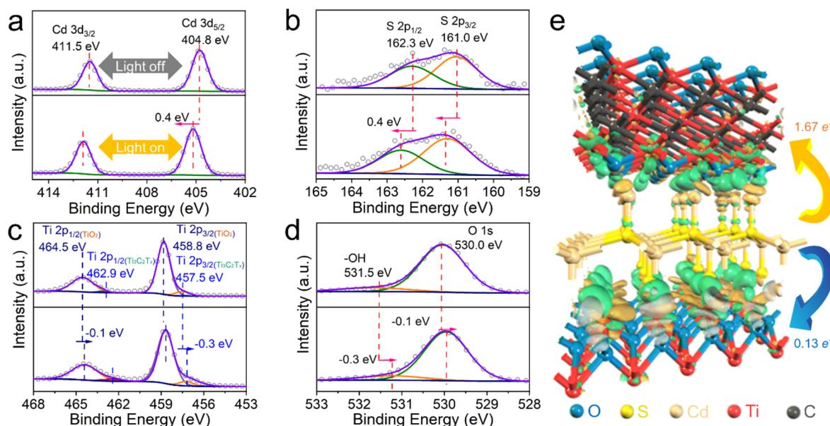
**Fig. 5** ISI-XPS characterization and DFT calculations of TC-0.1MX. (a) Cd 3d, (b) S 2p, (c) Ti 2p, and (d) O 1s XPS spectra in the dark (top) and under visible-NIR light irradiation of  $\lambda > 420$  nm (bottom). (e) The electron density difference of TC-MX. Forest green and yellow regions indicate accumulation and depletion of electrons, respectively.
