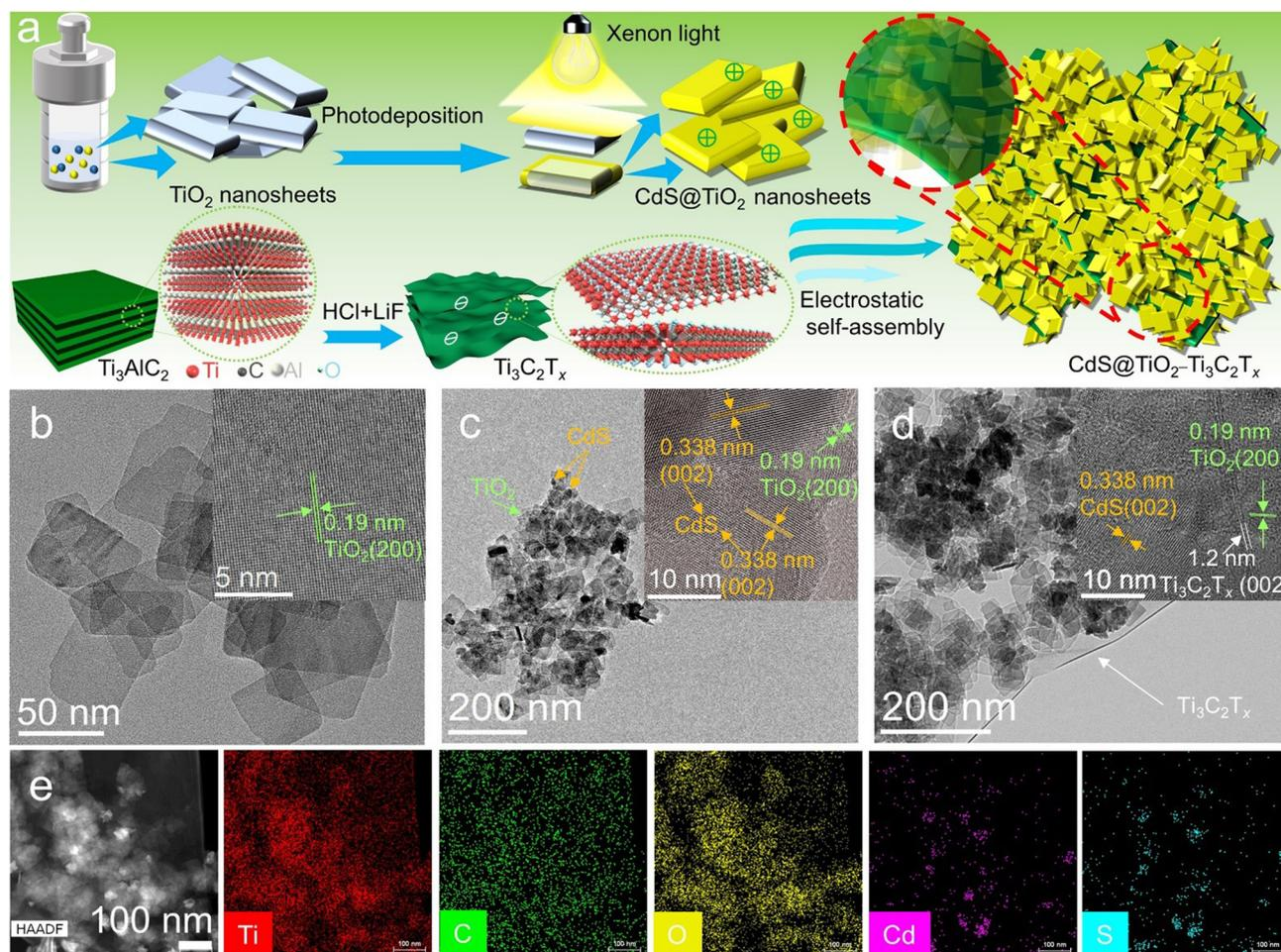
**Fig. 1** Fabrication of TC-MX ternary heterostructures. (a) Schematic illustration for the preparation of TC-MX ternary heterostructures. The morphologies and textural structures of the samples. TEM images of (b)  $\text{TiO}_2$ , (c) TC-2 and (d) TC-0.1MX; the insets are the corresponding HRTEM images. (e) HAADF-STEM image of TC-0.1MX with the corresponding Ti, C, O, Cd, and S EDX mapping results.
