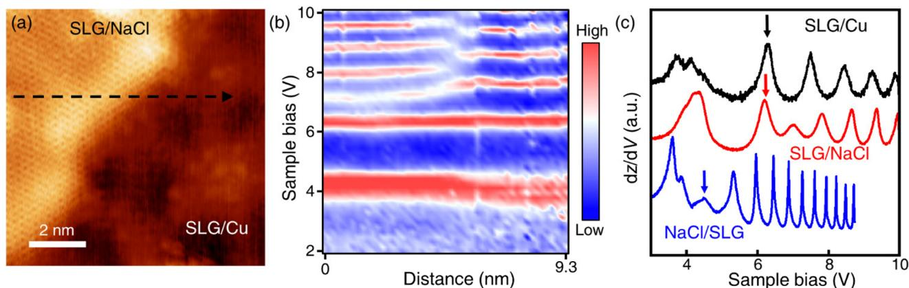
**Fig. 3** Variation in FER spectra owing to NaCl intercalation and adsorption. (a) STM topography image of SLG/Cu and NaCl-intercalated graphene ( $V_s = 50$  mV,  $I_t = 0.4$  nA). (b) 1D  $dz/dV$  map along the dashed arrow in (a). (c) FER spectra measured on the SLG/Cu (black), SLG/NaCl (red), NaCl/SLG (blue). FER peaks ( $n = 1$ ) are marked by arrows in (c).
