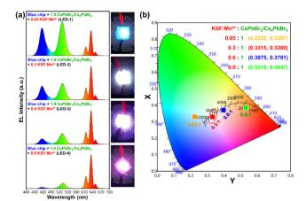
Fig. 9 (a) The electroluminescence spectra of the designed LED devices by varying the  $\rm K_2SiF_6:Mn^{4+}$  to  $\rm CsPbBr_3/Cs_4PbBr_6$  ratio in the wt% of 0.05:1, 0.3:1, 0.6:1, and 0.9:1 under forward-bias current of 20 mA (inset images are photographs of the working LEDs (LED 1–4), (b) the CIE chromaticity coordinates corresponding to the constructed LED devices using different composite wt% ratios.
