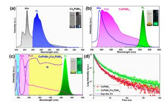
Fig. 5 (a) Absorption and photoluminescence spectra of pure Cs<sub>4</sub>PbBr<sub>6</sub>, (b) absorption, photoluminescence, and excitation spectra of pure CsPbBr3, (c) absorption, photoluminescence, and excitation spectra of dual-phase CsPbBr3/Cs4PbBr6, and (d) time-resolved photoluminescence decay curves of CsPbBr<sub>3</sub>, and CsPbBr<sub>3</sub>/Cs<sub>4</sub>PbBr<sub>6</sub> at  $\lambda_{\text{exci}}$  =
