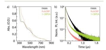
Fig. 3 (a) Absorption spectra for the FAMA perovskite thin film (black) and bilayer devices (RubDBP: pink, 1-CBPEA: green). (b) Perovskite PL decays for the FAMA and bilayer devices under 780 nm excitation at an excitation density of 44.2 mW cm<sup>-2</sup>. A 780 nm notch filter and an 800 nm long pass filter were used to remove laser scatter and isolate the perovskite emission.
