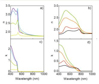
Fig. 4 The refractive index (a and b) and extinction coefficient (c and d) calculated for the ligand-free quantum dots of different composition and size. (a and c) MAPbBr $_3$  QDs (green line, QD size: 2.4 nm; blue line, 2.3 nm; violet line, 2.2 nm) and a polycrystalline film (yellow line). (b and d) MAPbI $_3$  QDs (red line, 9 nm; orange line, 7 nm; green line, 6 nm) and a polycrystalline film (black line).
