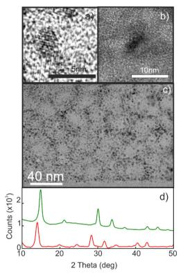
Fig. 1 (a and b) High-resolution TEM micrographs of MAPbBr<sub>3</sub> (a) and MAPbl<sub>3</sub> (b) nanocrystals inside a porous silica matrix. (c) The TEM cross section of the QD-MAPbBr3@SiO2 composite layer. (d) XRD diffractograms of QD-MAPbBr3@SiO2 (green line) and QD-MAPbl3@SiO2 (red line). For the sake of clarity, backgrounds were subtracted in both diffractograms.
