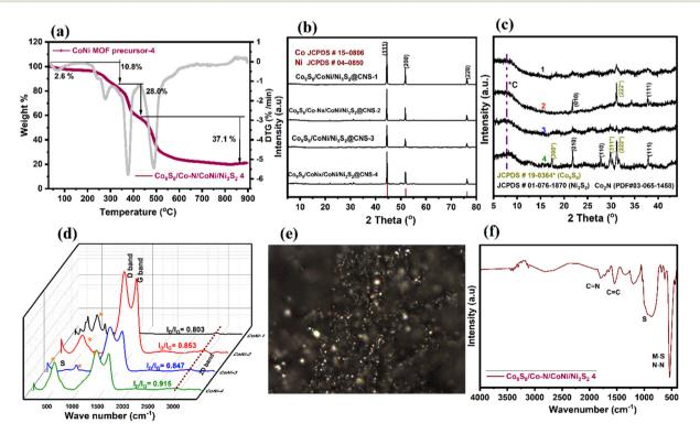
Fig. 4 (a) TGA spectrum of MOF precursor-4 conversion to catalyst  $Co_9S_8/Co-N_x/CoNi/Ni_3S_2@CNS-4$ , (b and c) XRD patterns of electrocatalysts  $CoS/Co-N_x/CoNi/NiS@CNS$ , (d) Raman spectra of catalysts 1–4, (e) Raman image (laser at 532 nm) of a filter showing the distribution of graphitic carbon, and (f) the FT-IR spectrum of  $Co_9S_8/Co-N_x/CoNi/Ni_3S_2@CNS-4$ .
