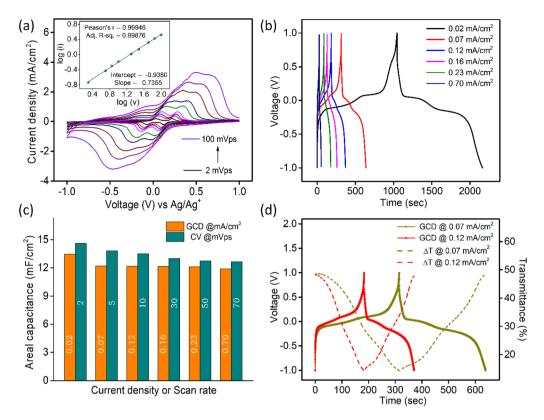
Fig. 3 (a) Scan rate dependent CV data and in the inset log(i) vs. log(v) plot, (b) GCD plots at different current densities, and (c) comparison of areal capacitances calculated from CV and GCD measurements, (d) in situ transmission data at 485 nm synchronized with the GCD data at different current densities.
