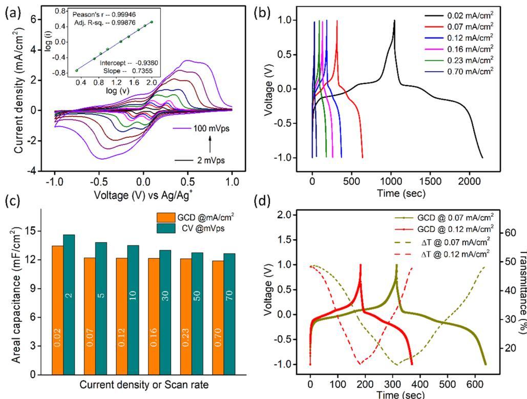
**Fig. 3** (a) Scan rate dependent CV data and in the inset  $\log(i)$  vs.  $\log(v)$  plot, (b) GCD plots at different current densities, and (c) comparison of areal capacitances calculated from CV and GCD measurements, (d) *in situ* transmission data at 485 nm synchronized with the GCD data at different current densities.
