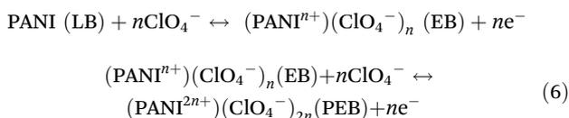
Two pairs of redox peaks arise in the CV profile of PANI due to the doping/dedoping of anions, as presented in Fig. S12.† The first redox couple at lower potentials is attributed to the transition between the LB and EB states and the second pair of
