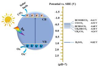
Fig. 1 Schematic diagram of photocatalytic  ${\rm CO_2}$  reduction over a semiconductor.
