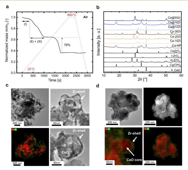
Fig. 3 (a) Weight loss of CaCO<sub>3</sub> nanoparticles containing a carbonaceous template coating during calcination in air (heating ramp of 25 °C min<sup>-1</sup> up to 900 °C), (b) XRD patterns of calcined zirconia-stabilized sorbents after template removal; TEM micrographs and EDX-TEM elemental maps for Ca and Zr for (c) a zirconia-stabilized, yolk-shell structured sorbent (Ca@12Zr) and (d) a zirconia-stabilized, core-shell-structured sorbent (Ca-26Zr).
