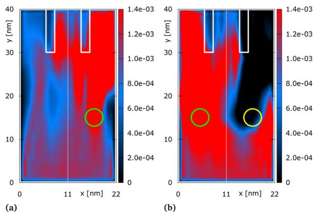
**Fig. 3** Distribution of quantum electron density [a.u.] for two asymmetric gate configurations:  $\phi_{G1} = 0$  V and  $\phi_{G2} = 0.21$  V (a) and  $\phi_{G1} = 0.21$  V and  $\phi_{G2} = -0.21$  V (b). The yellow circle indicates the location of the negatively charged gate.
