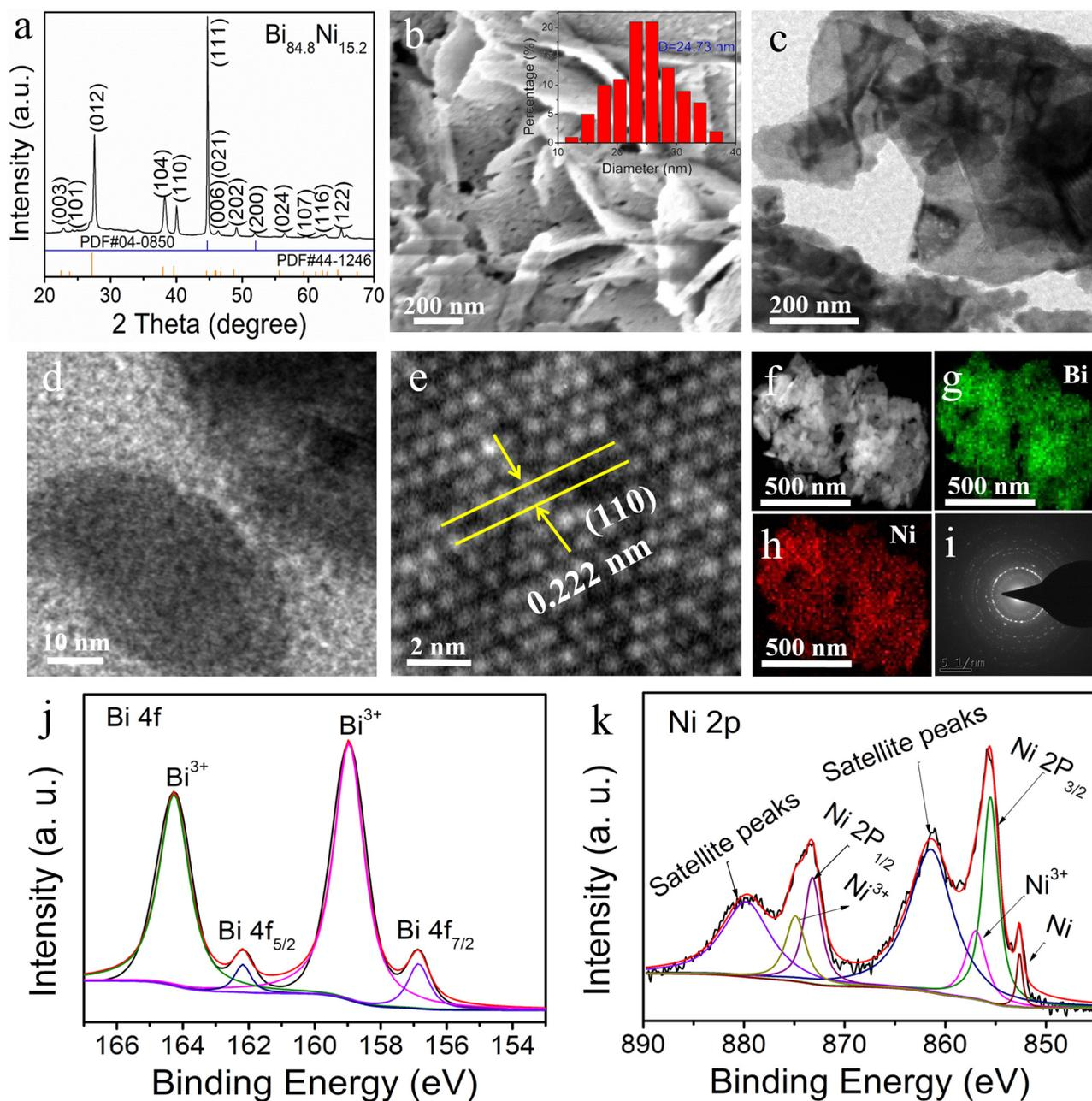
**Fig. 1** Characterizations of mesoporous  $\text{Bi}_{84.8}\text{Ni}_{15.2}$  alloy (a) XRD patterns; (b) SEM image; inset: pore-distribution image; (c and d) TEM images; (e) HRTEM image; (f) HAADF-STEM image; (g and h) EDS mapping images; (i) SAED pattern; (j) XPS spectrum of Bi 4f; (k) XPS spectrum of Ni 2p.
