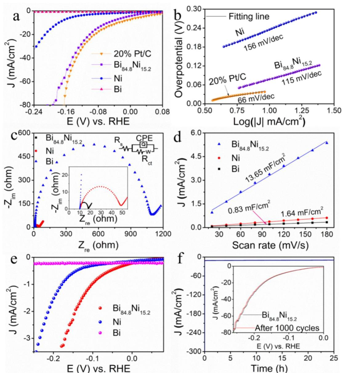
**Fig. 2** (a) Polarization curves of samples for HER in 1.0 M KOH; (b) Tafel plots; (c) Nyquist plots at  $-56$  mV vs. RHE. Inset shows the equivalent circuit; (d) capacitive current as a function of scan rate for the samples; (e) specific activity; (f)  $I-t$  test for  $\text{Bi}_{84.8}\text{Ni}_{15.2}$  alloy at  $-56$  mV vs. RHE; inset shows the polarization curves at  $5$  mV  $\text{s}^{-1}$  before and after 1000 cycles of CV.
