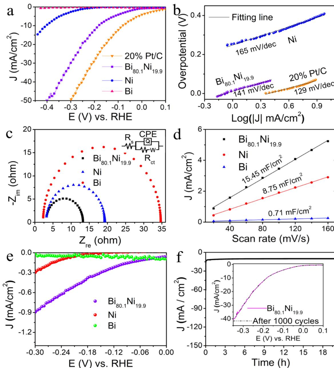
**Fig. 3** (a) Polarization curves for HER in 1.0 M PBS (pH 7.0); (b) Tafel plots; (c) Nyquist plots at  $-183$  mV vs. RHE. Inset shows the equivalent circuit; (d) capacitive current as a function of scan rate for the samples; (e) specific activity; (f)  $I-t$  test for  $\text{Bi}_{80.1}\text{Ni}_{19.9}$  alloy at  $-183$  mV vs. RHE; inset shows the polarization curves at  $5$  mV  $\text{s}^{-1}$  before and after 1000 cycles CV.
