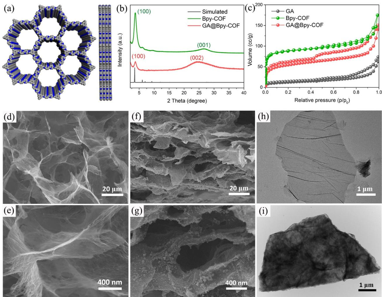
**Fig. 1** (a) Space-filling packing diagram of Bpy-COF from different views. (b) PXRD patterns of the pristine Bpy-COF and GA@Bpy-COF. (c)  $N_2$  sorption isotherms of the GA, Bpy-COF and GA@Bpy-COF. (d and e) SEM images of the GA. (f and g) SEM images of the GA@Bpy-COF. TEM images of (h) graphene and (i) the GA@Bpy-COF.
