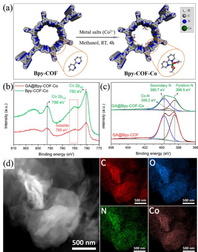
**Fig. 2** (a) Schematic illustration of the fabrication of GA@Bpy-COF-Co. (b) Co 2p XPS spectra of GA@Bpy-COF-Co and Bpy-COF-Co. (c) N 1s XPS spectra of GA@Bpy-COF-Co and the GA@Bpy-COF. (d) HAADF-STEM images with the corresponding elemental mappings of C, O, N, and Co.
