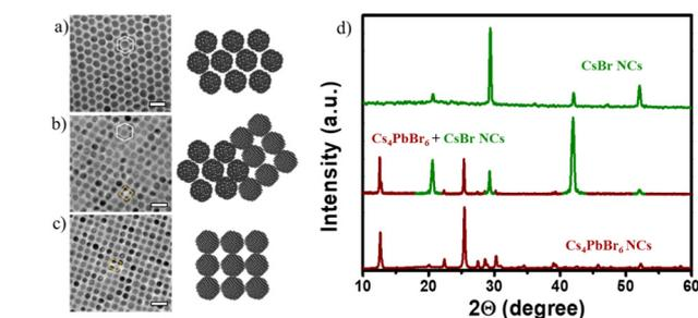
**Fig. 5** (a–c) TEM images of NCs with two different packings (hexagonal close packing, HCP, and cubic close packing, CCP) while the reaction condition was transferring from  $\delta_2$  to  $\delta_3$ . Scale bars are 20 nm in all the images. (d) Powder XRD patterns of the samples in the regions of  $\delta_2$  and  $\delta_3$  corresponding to  $\text{Cs}_4\text{PbBr}_6$  and  $\text{CsBr}$  NCs along with their mixed region.
