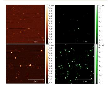
Fig. 4 AFM (A and C) and conductive AFM (B and D) images of the NIP (A and B) and MIP (C and D) films after a 30 s electrodeposition of gold from a 0.2 mM HAuCl<sub>4</sub> solution.
