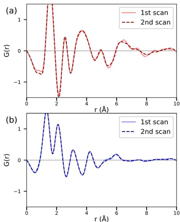
**Fig. 4** Area-averaged STEM-ePDF profiles for two scans of the same area for (a) the  $0.67[(\text{Na}_2\text{O})_{10.9}(\text{P}_2\text{O}_5)]-0.33[(\text{AlO}_{3/2})[\text{AlF}_3]_{1.5}]$  inorganic glass and (b)  $a_g\text{ZIF-62}$ . The grey horizontal lines mark zero on the vertical axes.
