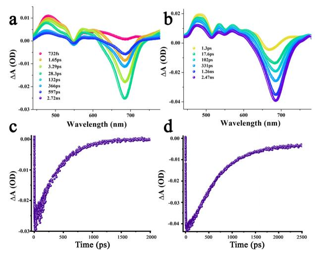
Fig. 9 fs-TA spectra at the indicated delay time of (a) ZnP-azaBDP dyad 6, and (b) H<sub>2</sub>P-azaBDP dyad 5, in o-DCB. The samples were excited at 424 nm. The profile of the 682 nm peak corresponding to <sup>1</sup>azaBDP\* in the ZnP-azaBDP dyad 6 and the H<sub>2</sub>P-azaBDP dyad 5 is shown in (c) and (d), respectively.
