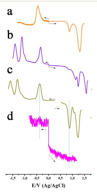
Fig. 7 DPVs of azaBDP 4 (orange),  $H_2P$ -azaBDP dyad 5 (purple), ZnP-azaBDP dyad 6 (olive) and (ZnP-azaBDP)-graphene hybrid 11 (pink), in o-DCB containing 0.1 M (TBA)ClO $_4$  as the electrolyte.
