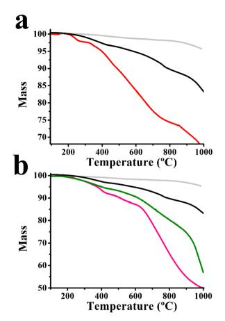
Fig. 3 Thermograms of (a) few layered graphene (grey), 7 (black) and 9 (red), and (b) few layered graphene (grey), 7 (black), 10 (green) and 11 (pink), obtained under  $N_2$ .
