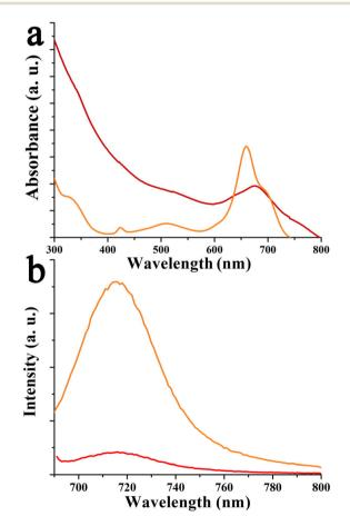
Fig. 5 (a) Absorption and (b) fluorescence spectra ( $\lambda_{\rm exc}$  686 nm) of 4 (orange) and 9 (red), in o-DCB.
