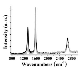
Fig. 2 Raman spectra (633 nm) of few layered graphene (grey) and material 7 (black), normalized at the G band.
