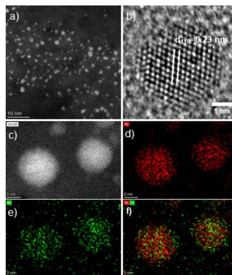
**Fig. 3** HAADF-STEM analysis of intermetallic PdIn NPs and elemental distribution: (a) representative HAADF-STEM image, (b) atomic-resolution HRTEM image of an individual PdIn NP. (c) HAADF-STEM image of PdIn NPs and corresponding EDS elemental mapping of (d) Pd, (e) In, and (f) Pd + In.
