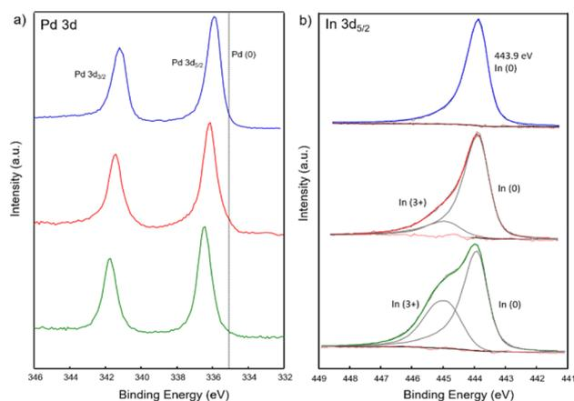
**Fig. 4** (a) Pd 3d and (b) In 3d<sub>5/2</sub> XPS spectra of PdIn (red), Pd<sub>3</sub>In (blue) and Pd<sub>3</sub>In<sub>7</sub> (green) NPs.
