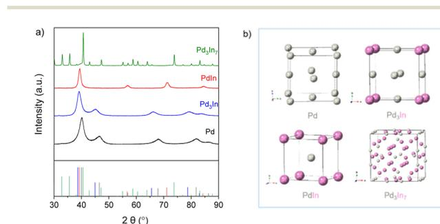
**Fig. 1** (a) X-ray diffraction patterns and (b) illustration of the unit cell and crystal structures of the L<sub>10</sub> Pd<sub>3</sub>In, B2 PdIn and Pd<sub>3</sub>In<sub>7</sub> phase (references: Pd<sub>3</sub>In<sub>7</sub> (green, ICDD 98-040-8314), PdIn (red, ICDD 98-005-9473), Pd<sub>3</sub>In (blue, ICDD 98-024-7193), Pd (black, ICDD 98-004-1517)).
