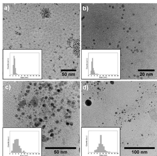
**Fig. 2** TEM images with particle size distribution of (a) Pd NPs, (b) Pd<sub>3</sub>In NPs, (c) PdIn NPs, and (d) Pd<sub>3</sub>In<sub>7</sub> NPs.
