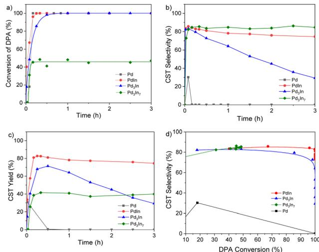
Fig. 6 Catalytic performance of Pd@IL, Pd<sub>3</sub>In@IL, PdIn@IL, and Pd<sub>3</sub>In<sub>7</sub>@IL in the selective hydrogenation of diphenylacetylene (reaction conditions: 80 °C, 10 bar H<sub>2</sub>, Pd–In NPs@IL, 30 ml THF, 5.6 mmol DPA): (a) conversion, (b) CST selectivity, (c) CST yield over reaction time and (d) CST selectivity over DPA conversion.
