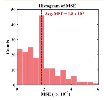
Fig. 5 Statistical analysis of MSE over the test dataset (for the forward trained model). This MSE histogram shows that 96% of the test samples have an MSE  $<4.2 \times 10^{-3}$ .
