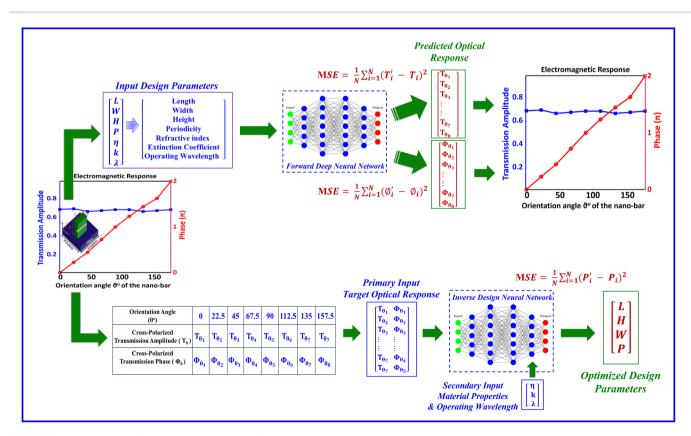
Fig. 2 Structural outline of the proposed forward and inverse design models.
