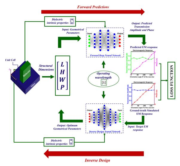
Fig. 1 A pictorial representation of the proposed forward and inverse design models. The forward predicting network takes the structural dimensions, dielectric intrinsic properties and operating wavelength as the input and predicts the cross-polarized transmission amplitude and phase. The inverse model takes the target EM response as the input, along with the material and desired wavelength specifications as the input, to predict optimum geometrical parameters as the output.
