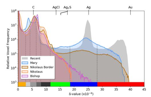
Fig. 7 Comparison between the delta value histograms of the samples *Nicolaus Border*, *Nicolaus, Bishop* and *Mary*, together with the *Recent* histogram for a comparison to modern Zwischgold. The data has been median-filtered in order to decrease peak widths and the histograms have been scaled to normalise against different sample sizes. The colour bar along the lower edge indicates the segmentation for the PXCT 3D model presentations shown in other figures.
