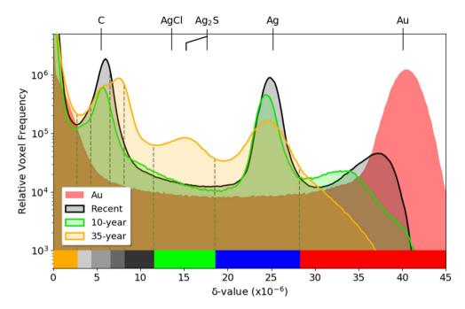
Fig. 3 Comparison between the PXCT  $\delta$ -value histograms of the *Recent*, 10-year, and 35-year samples and a pure gold reference. The histograms have been scaled to match the average number of total voxels with a  $\delta$ -value above 3  $\times$  10<sup>-6</sup> in order to normalise against different sample sizes. The colour bar along the lower edge indicates the segmentation for the PXCT tomogram presentations shown in other figures.
