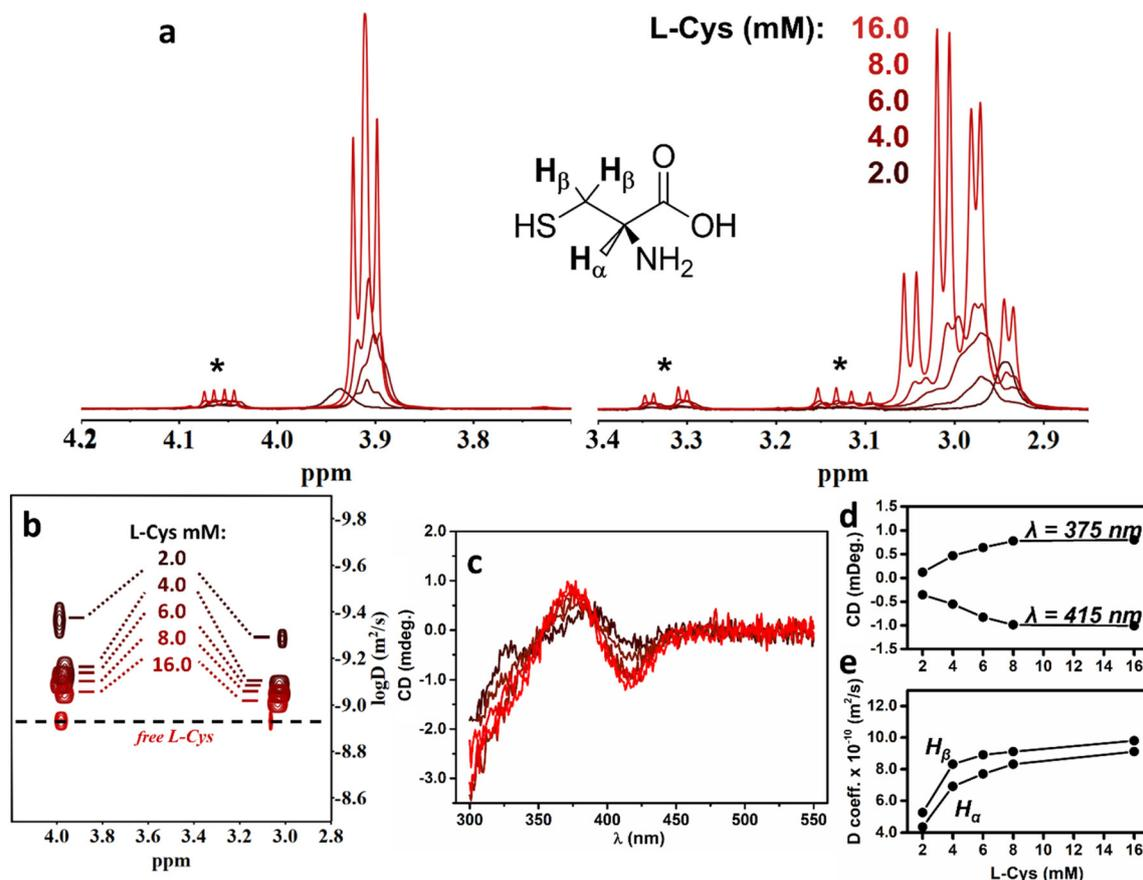
**Fig. 4** (a)  $^1\text{H-NMR}$  titration spectra of a  $1\text{ mg ml}^{-1}$  solution of L-AIS QDs with different L-Cys concentrations, the signals that are ascribed to L-cystine are marked with an asterisk. (b) DOSY and (c) CD spectra of L-AIS QD solutions in the presence of different L-Cys concentrations. (d and e) Plots of the intensity of the CD bands and the measured diffusion coefficients respectively.
