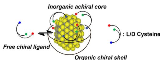
Fig. 5 Schematic representation on the ligand–nanoparticle chiral hybrid structure.
