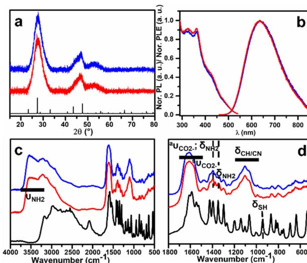
Fig. 2 Chemico-physical characterization of L-AIS (blue) and D-AIS (red) QDs: (a) XRD patterns; reference pattern: cubic  $\text{AgIn}_5\text{S}_8$ , ICSD 51619. (b) PLE and PL spectra of the QD solutions. (c and d) FTIR spectra of the QD powders and the reference spectra for zwitterionic L-Cys (black).
