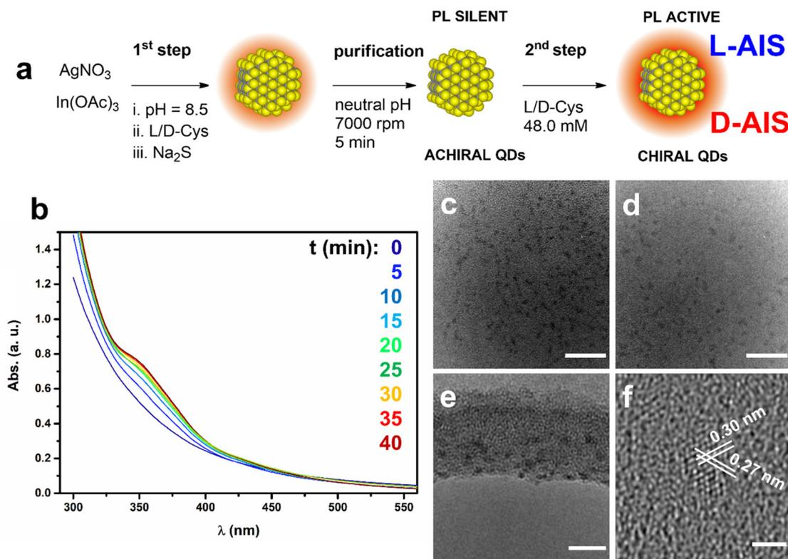
**Fig. 1** (a) Schematic representation of the synthesis. (b) UV/Vis analysis of the reaction mixture at different reaction times. (c) TEM micrographs of non-stoichiometric AIS QDs with scale bars: (c and d) = 20.0 nm, (e) = 10.0 nm and (f) = 2.0 nm.
