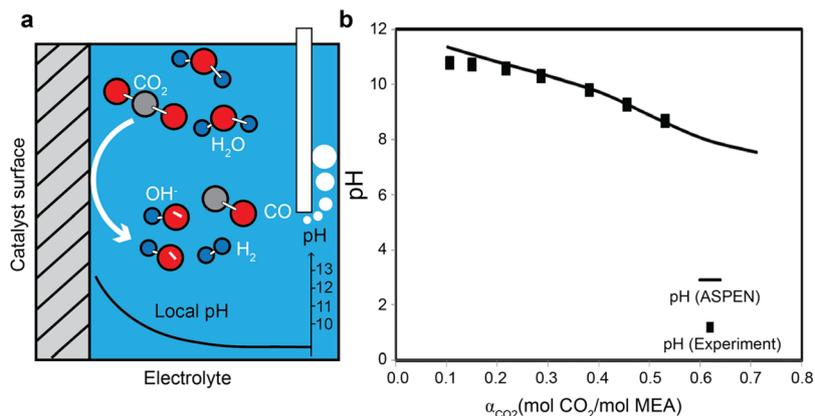
**Fig. 4** (a) A schematic illustration of local pH difference for gas-fed CO<sub>2</sub> electroreduction close to the catalyst surface. (b) The pH evolution as a function of CO<sub>2</sub> loading in 30 wt% MEA aqueous solution at 21 °C. Reproduced with permission,<sup>54</sup> copyright 2012, American Chemical Society.
