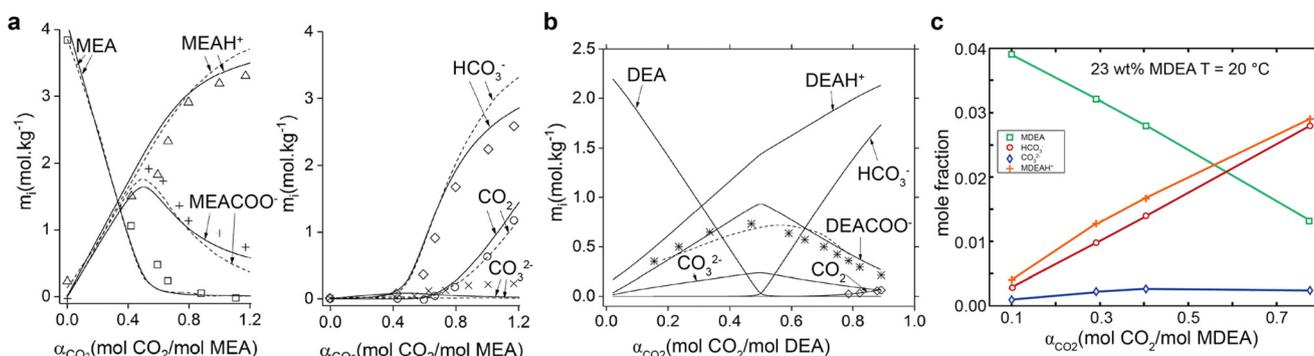
**Fig. 2** Evolution of chemical species in the monoethanolamine-CO<sub>2</sub>-H<sub>2</sub>O system in (a) 20 wt% MEA at 40 °C, (b) 20 wt% DEA at 25 °C with symbols for experimental results and lines for calculated values (reproduced with permission,<sup>46</sup> Copyright 2018, American Chemical Society), (c) 23 wt% MDEA aqueous solution at 20 °C. Reproduced with permission.<sup>44</sup> Copyright 2005, American Chemical Society.
