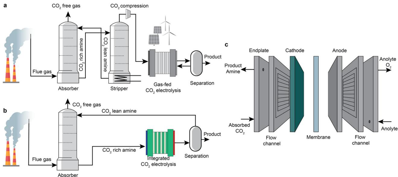
**Fig. 1** Schematic illustration of (a) sequential CO<sub>2</sub> capture and electrolysis based on gas-fed electrolyzers, (b) an integrated route based on integrated electrolyzers, and (c) cell configuration of a single cell of the integrated electrolyzers.
