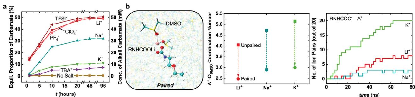
**Fig. 11** (a) Comparison of equilibrium population and concentration of alkali and tetrabutylammonium (TBA<sup>+</sup>) cations in CO<sub>2</sub>-loaded 0.1 M EEA in DMSO. (b) A Li-carbamate pairing configuration solvated in DMSO (left) and molecular dynamics simulation results in alkali cations coordination numbers (middle) and the number of ion pairs formed against computation time (right). Reproduced with permission,<sup>69</sup> copyright 2019, American Chemical Society.
