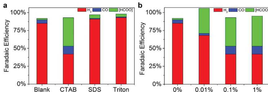
**Fig. 12** Product distributions of CO<sub>2</sub> reduction over indium catalyst at –0.8 V vs. RHE in CO<sub>2</sub>-saturated 30 wt% MEA aqueous solution with (a) 0.1 wt% of CTAB, sodium dodecyl sulfate (SDS), and Triton surfactants, and (b) with different concentrations of CTAB surfactant. Reproduced with permission,<sup>60</sup> copyright 2017, John Wiley and Sons.
