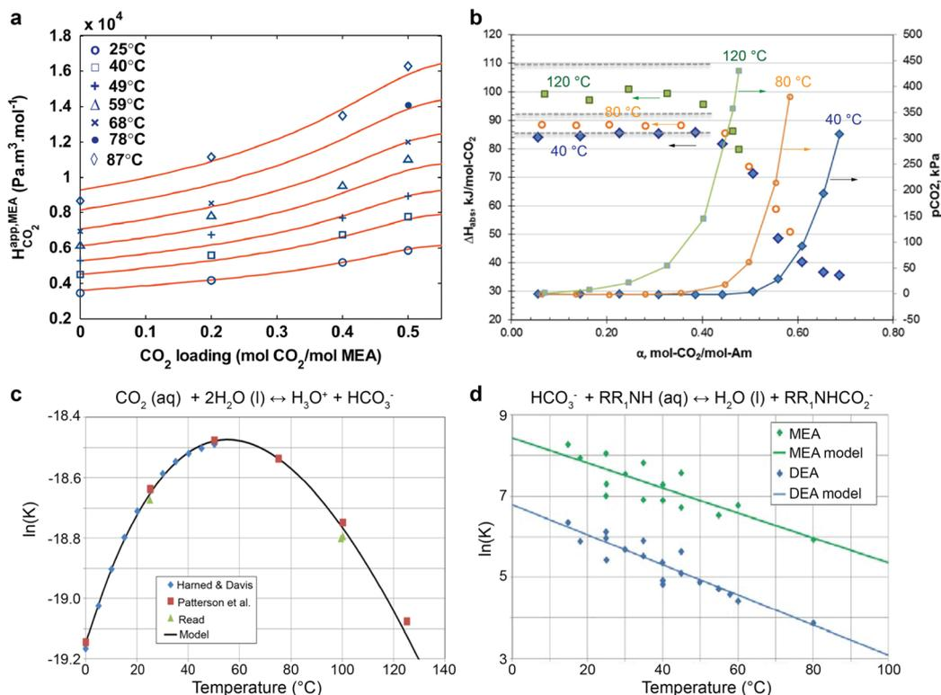
**Fig. 3** The temperature effects on (a) Henry constant of CO<sub>2</sub>, reproduced with permission,<sup>49</sup> copyright 2011, Elsevier. (b) CO<sub>2</sub> partial pressure and heat of CO<sub>2</sub> absorption for 30 wt% MEA aqueous solutions, reproduced with permission,<sup>50</sup> copyright 2014, Elsevier, (c) bicarbonate formation, and (d) carbamate formation for MEA and DEA aqueous solution. Reproduced with permission,<sup>51</sup> copyright 2017, Elsevier.
