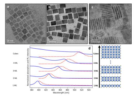
Fig. 1 TEM and spectroscopy of nanocubes and NPLs. TEM micrographs of CsPbBr<sub>3</sub> nanocubes (a) and NPLs (b and c). Absorption (solid blue lines) and emission (dashed red lines) spectra of ensembled CsPbBr<sub>3</sub> NCs, corresponding to 1, 2, 3, 4 ML and cubes (d).
