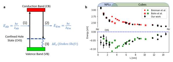
Fig. 4 (a) Schematically energetic ordering of relevant absorption and emission transitions within CsPbBr<sub>3</sub> NCs (a). Size-dependent NC emission and absorption with theoretical calculation of CBES and VBES energies, plotted relative to CHS energies, which are set to zero (b).
