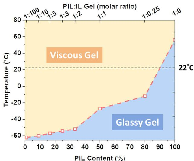
**Fig. 3** The phase diagram of PIL:IL mixture (in molar ratio) measured by DSC, with a scanning rate of  $10\text{ }^{\circ}\text{C min}^{-1}$  under  $\text{N}_2$ . The glass transition ( $T_g$ ) points are connected with red dashed line as the hypothetical trend of phase-transition of the gel from the glassy state to elastomeric state. The plot of DSC curve from which  $T_g$  was obtained is given in Fig. S6.†
