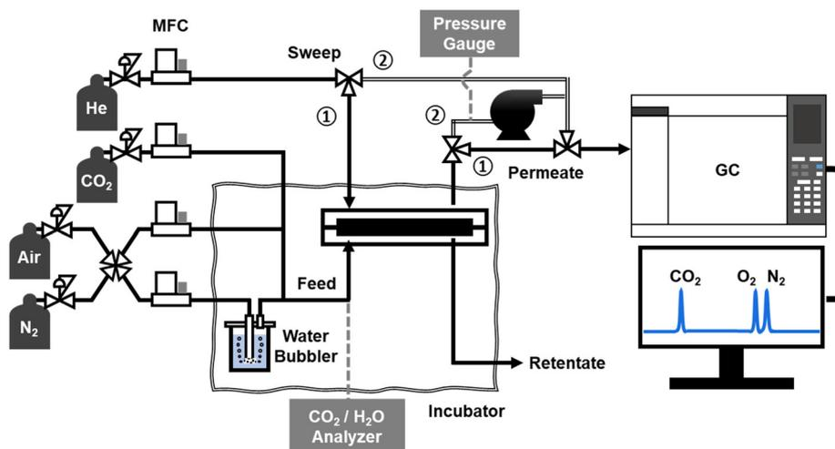
**Fig. 1** Schematics of the membrane test unit. Permeate gas was collected and sent to gas chromatogram (GC) either by He sweep (path ①) or by vacuum (path ②) for a transmembrane pressure of 0 or 1 atm, respectively. The balance gas of CO<sub>2</sub> is either synthetic air (N<sub>2</sub>/O<sub>2</sub> = 80/20) or N<sub>2</sub> for the CO<sub>2</sub>/N<sub>2</sub>/O<sub>2</sub>/H<sub>2</sub>O or CO<sub>2</sub>/N<sub>2</sub>/H<sub>2</sub>O mixtures, respectively.
