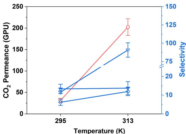
**Fig. 9** Performance of vacuum operation of PIL-IL/GO on bPES/PET (v in Table 1) under 410 ppm CO<sub>2</sub> with mixture feed of CO<sub>2</sub>/N<sub>2</sub>/O<sub>2</sub> at 22 and 40 °C; both with 40% RH.
