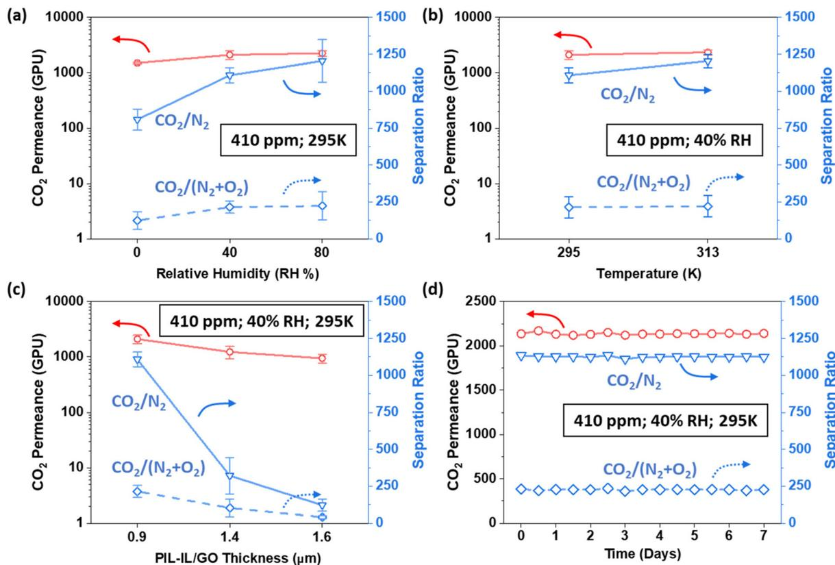
**Fig. 8** The change in CO<sub>2</sub> separation performance with humidity (a), temperature (b), membrane thickness (c), and time (d). Membrane ii (in Table 1) is used in panel (a), (b), and (d); and membrane ii, iii, and iv are used in panel (c).
