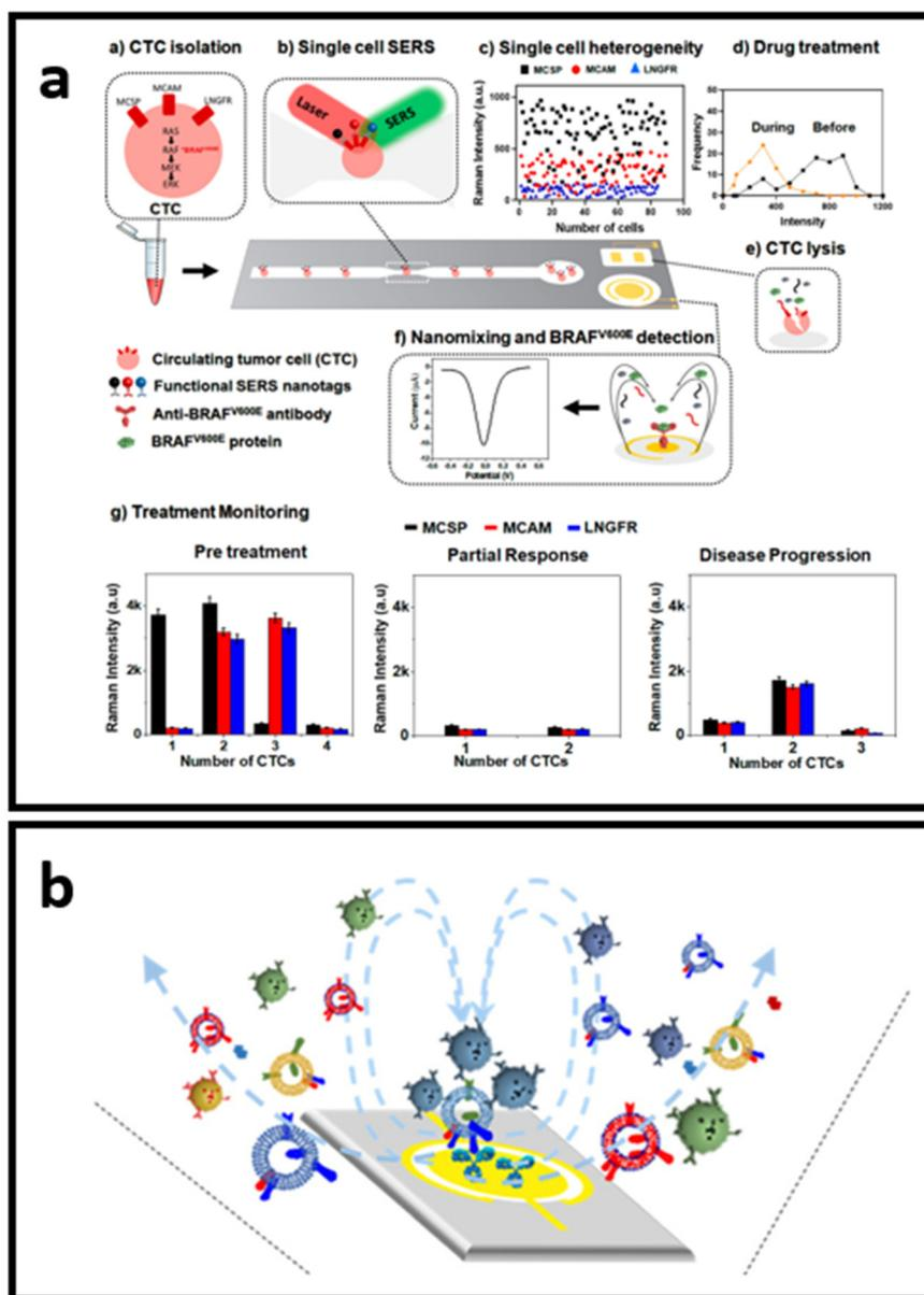
**Fig. 11** Schematics of the small devices with SERS-based sensors: (a) SERS-based microfluidic immunoassay for *in situ* characterization of single CTCs, adapted from ref. 214 with permission from the American Chemical Society, copyright 2021; (b) nano-mixing-enhanced EVs subpopulation characterization platform adapted from ref. 215 with permission from the American Chemical Society, copyright 2021.
