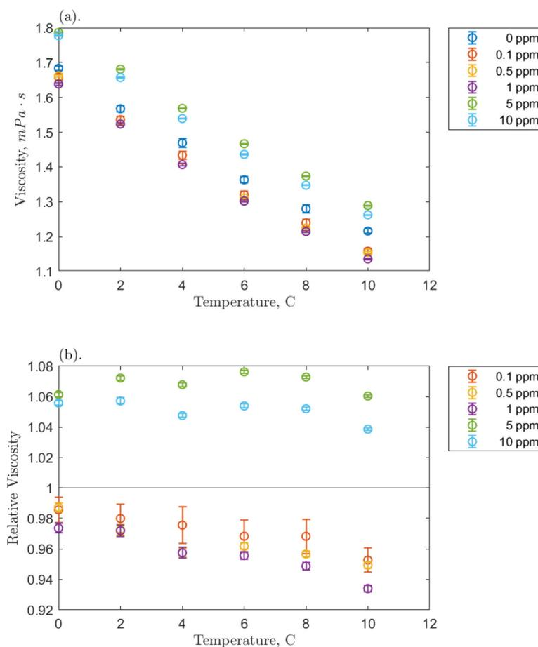
**Fig. 2** Temperature effect on the measured viscosity of the O-MWCNT–water system studied. This includes (a) the absolute viscosity and (b) the relative viscosity compared to a pure water baseline. Bars represent the 95% confidence intervals on the data, which are very small.
