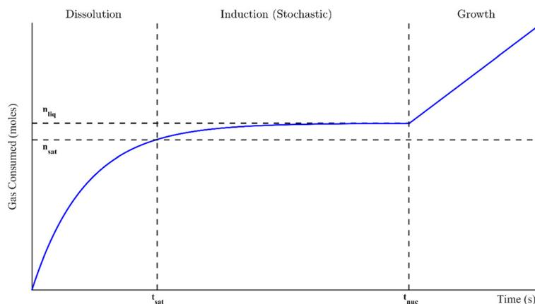
**Fig. 1** Schematic of a typical hydrate formation profile through guest gas consumption. Here,  $n_{\text{sat}}$  is the molar saturation value that occurs at  $t_{\text{sat}}$  and  $n_{\text{liq}}$  is the final number of moles in the supersaturated solution at nucleation, which occurs at  $t_{\text{nuc}}$ .
