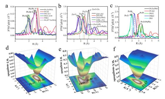
Fig. 6 FT  $K^2$ -weighted XANES spectra of (a) Pb and (b) Zn and the (c)  $Pt^{IV}$  K-edge radial distance spectra  $\chi(R)$  for three OIP QDs, as well as the references of Pb foil, PbO, PbO<sub>2</sub>, PbBr<sub>2</sub>, Zn foil, ZnBr<sub>2</sub>, ZnO, Pt foil, PtO<sub>2</sub>, PtBr<sub>2</sub> and PtO at the K-edge. Wavelet transform extended X-ray absorption fine structure (WTEXAFS) of  $Pt^{IV}$ /Zn/PbO/PC-Zn/MAPbBr<sub>3</sub> for (d) Pb, (e) Zn and (f)  $Pt^{IV}$ .
