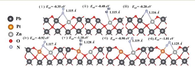
Fig. 7 Adsorption energy and the bond length of  $N_2$  absorbed on the surface of Zn-doped (i, ii and iii) and  $Pt^{IV}/Zn$  co-doped (iv, v and vi) catalysts in both end-on and side-on configurations. The interactions between the oxygen vacancy and Pb, Pt and Zn were examined.
