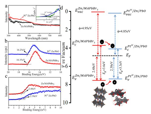
Fig. 5 Band structures of  $Pt^{IV}/Zn/PbO/PC-Zn/MAPbBr_3$ . (a) The calculations of the optical band gap. (b) UPS spectra. (c) VBXPS spectra. (d) Schematic energy band diagram of the  $Pt^{IV}/Zn/PbO/PC-Zn/MAPbBr_3$  heterojunction.
