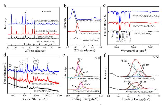
Fig. 2 Chemical characterization of PbO/PC-MAPbBr<sub>3</sub>, Zn/PbO/PC-Zn/MAPbBr<sub>3</sub> and Pt<sup>IV</sup>/Zn/PbO/PC-Zn/MAPbBr<sub>3</sub>. (a) XRD patterns. Dotted lines are the sectional PbO characteristic patterns. (c) FTIR spectra. (d) Raman spectra. XPS spectra of C 1s (e) and Br 3d (f) for Pt<sup>IV</sup>/Zn/PbO/PC-Zn/ MAPbBr<sub>3</sub> with and without etching.
