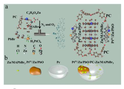
Scheme 1 The preparation of the  $Pt^{IV}$ /Zn/PbO/PC-Zn/MAPbBr<sub>3</sub> heterojunction materials. (a) A schematic illustration of the ESI-based microdroplet synthesis. (b) A schematic image of the structure.
