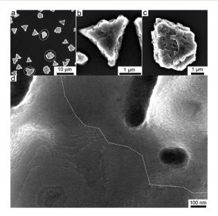
Fig. 21 (a) SEM image of AgNPs superlattices formed on the cathode at 400 V cm<sup>-1</sup>, showing faceted colloidal crystals. SEM images of AgNPs colloidal crystals with (b) triangular prism and (c) truncated triangular prism shapes. (d) High-resolution SEM image showing the preferential orientation of superlattices and a grain boundary highlighted with white dashed lines. Reprinted with permission from ref. 185 (copyright 2017, American Chemical Society).
