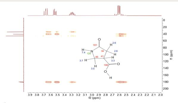
Fig. 1  $^{1}$ H $^{-13}$ C HMBC spectra taken in D<sub>2</sub>O and the chemical structure with NMR assignments of 1 (5-oxopyrrolidine-3-carboxylic acid) isolated from CD dialysate. Chemical shifts of proton, carbon and nitrogen are labeled in blue, red and green, respectively.
