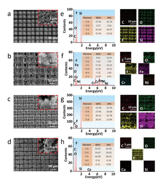
Fig. 2 (a-d) SEM images of quartz glass, stainless steel, silicon wafer, and paper after femtosecond laser ablation; (e-h) EDS spectra and elemental mapping of laser-treated quartz glass, stainless steel, silicon wafer, and paper, respectively.
