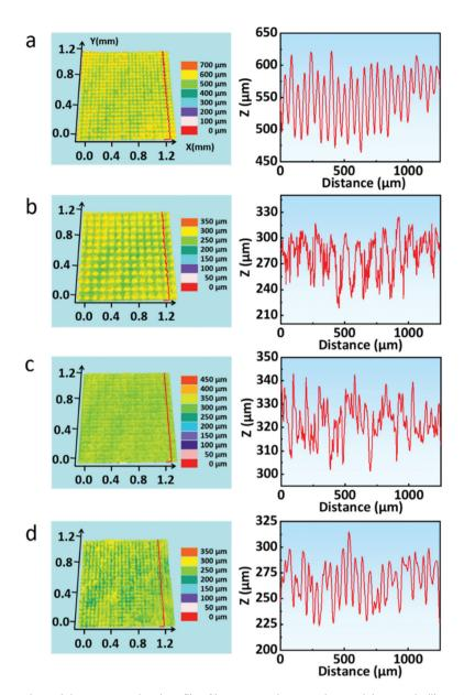
Fig. 3 (a-d) 3D surface topography and the cross-sectional profile of laser-treated quartz glass, stainless steel, silicon slice, and paper, respectively.
